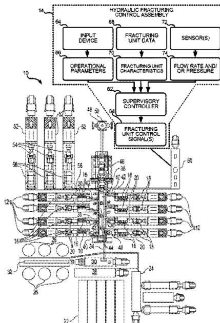
event and/or a pulsation event. The supervisory controller may be configured to generate a cavitation notification signal indicative of detection of cavitation associated with operation of the hydraulic fracturing pump, and/or a pulsation notification signal indicative of detection of pulsation associated with operation of the hydraulic fracturing pump.
