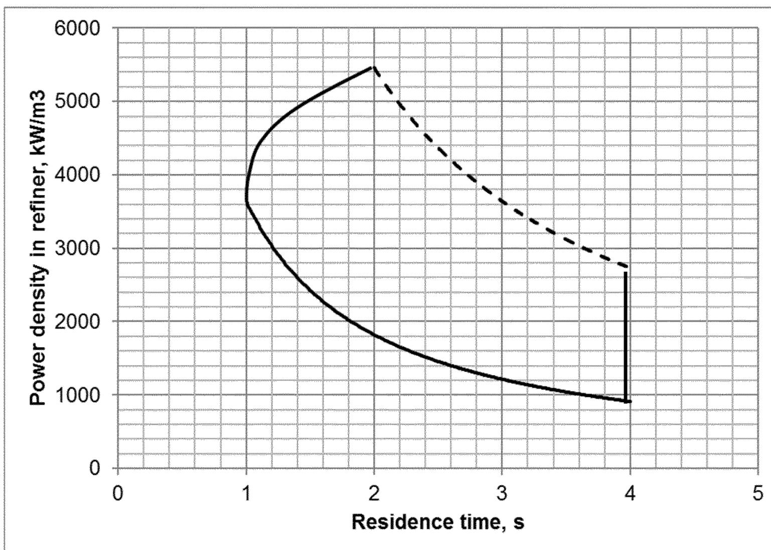
Fig. 8. A preferred range of power density vs. residence time in the refiner.
