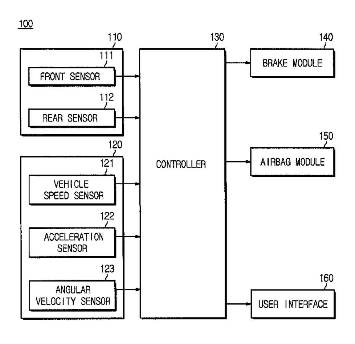
the forward collision and the rear-end collision, and control the brake module based on the target forward collision speed and the target rear-end collision speed.
