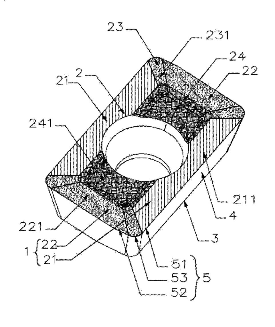
surface intersects the side surface to form the main cutting edge, the secondary cutting surface intersects the side surface to form the secondary cutting edge, a main coating is provided on the main cutting surface, a secondary coating is provided on the secondary cutting surface, and the main coating and the secondary coating are independent from each other.
