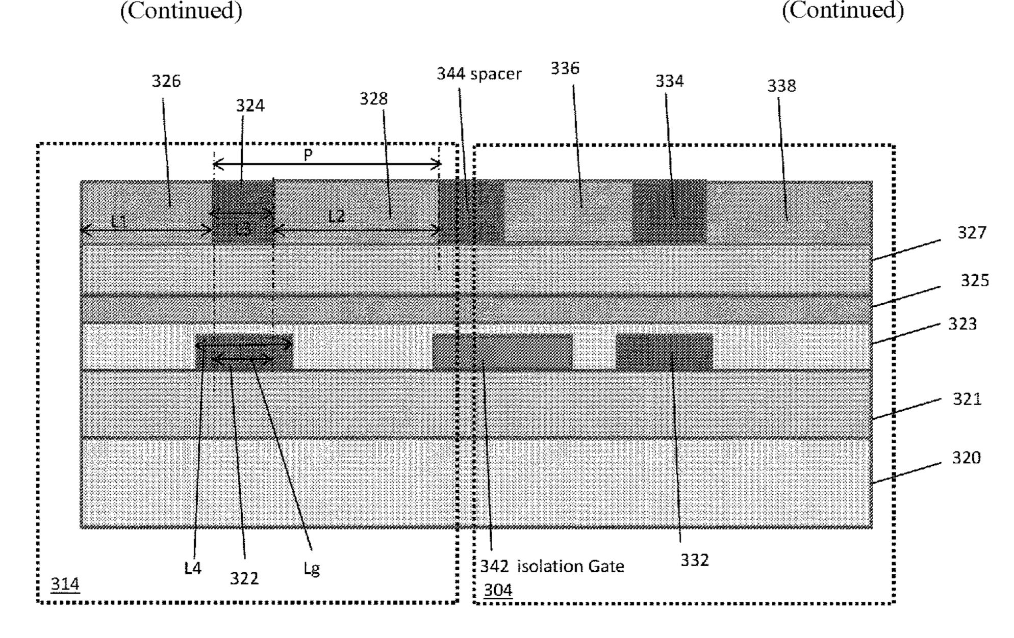
the gate length of the gate electrode may be determined by the spacer width. Other embodiments may be described and/or claimed.
