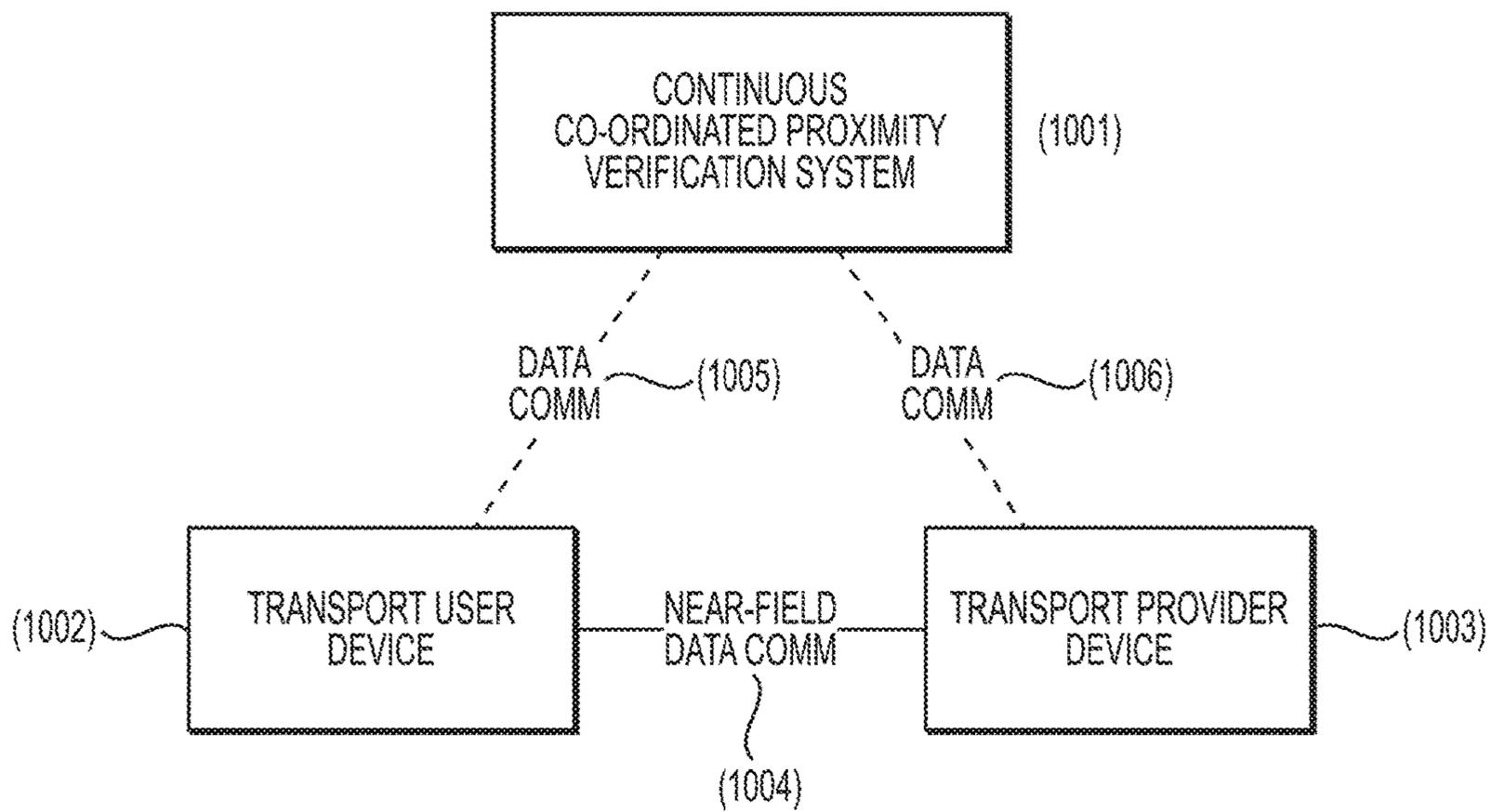
FIGURE 11b. METHOD 2 OF CONTINUOUS CO-ORDINATED PROXIMITY VIA VERIFICATION OF NEAR-FIELD COMMUNICATIONS LINK
