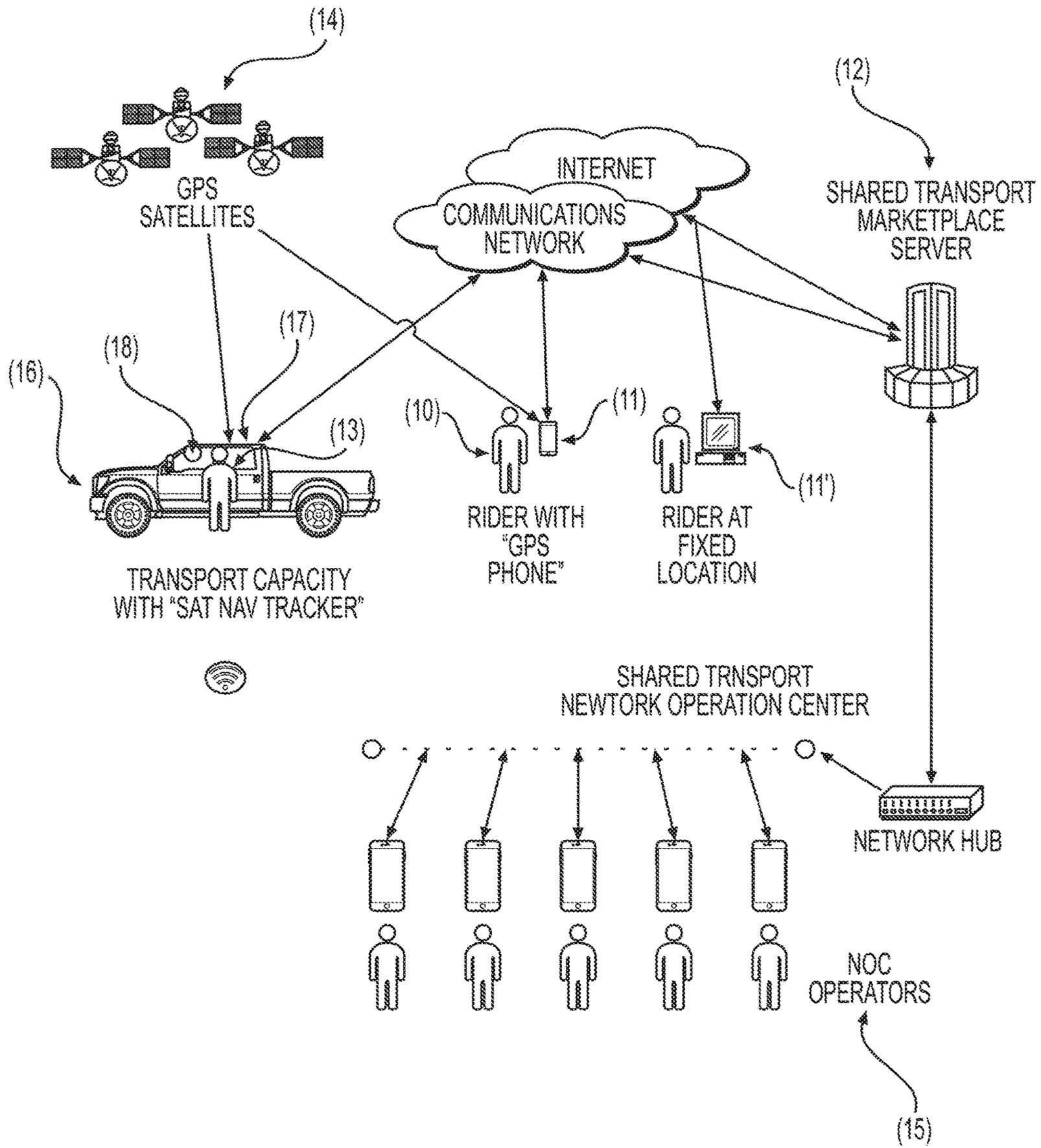
FIGURE 2. TRANSPORT CAPACITY COMPUTING AND COMMUNICATIONS COMPONENTS
