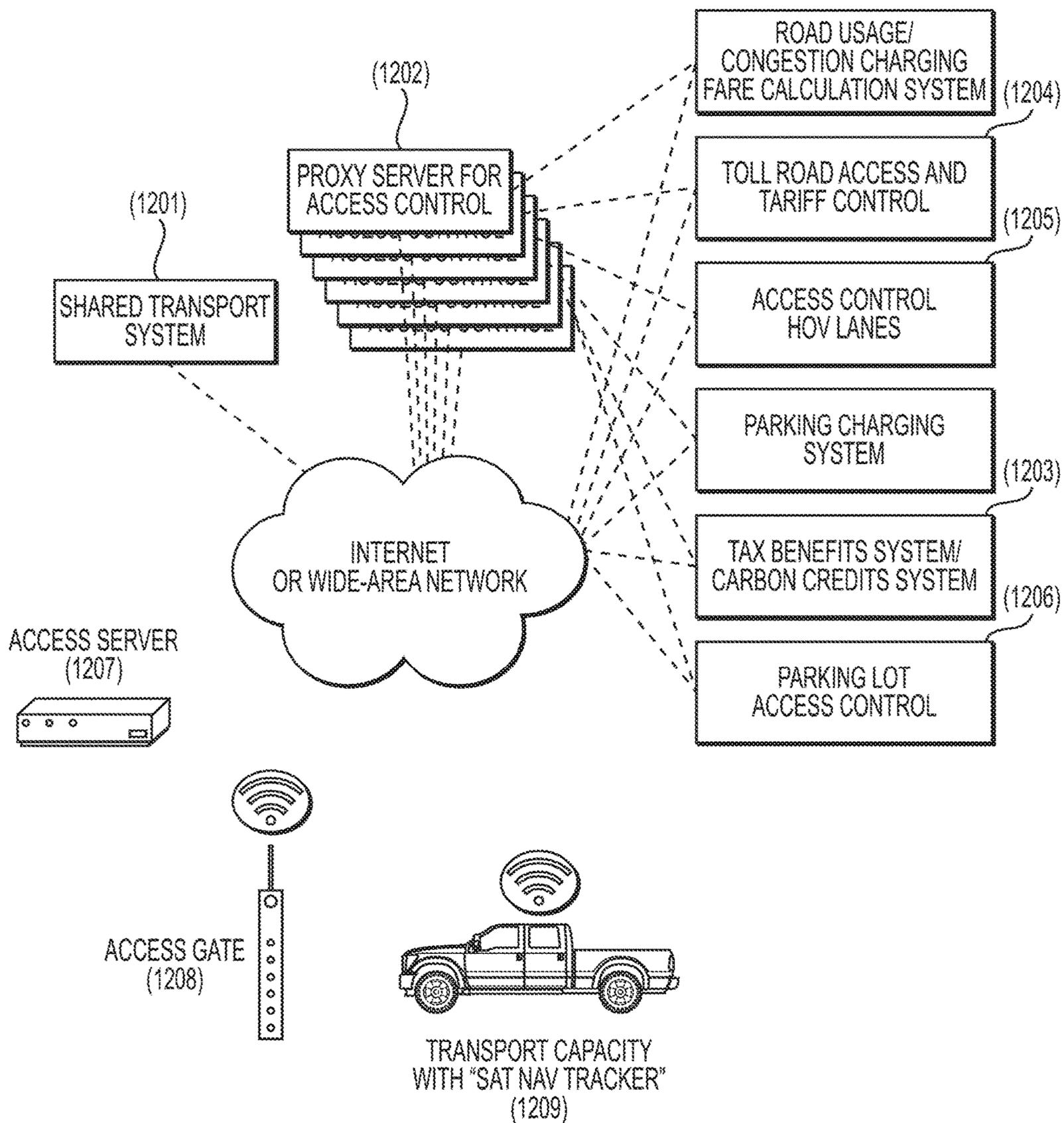
FIGURE 12b. ACCESS CONTROL SYSTEM, SERVER PUSH METHOD, SERVER-SIDE LOGIC
