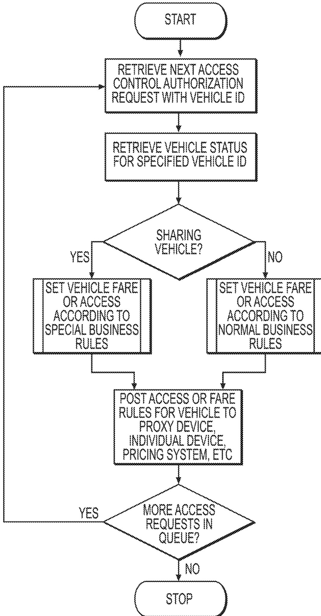
FIGURE 12e. ACCESS CONTROL SYSTEM, CLIENT PULL METHOD, CLIENT-SIDE LOGIC
