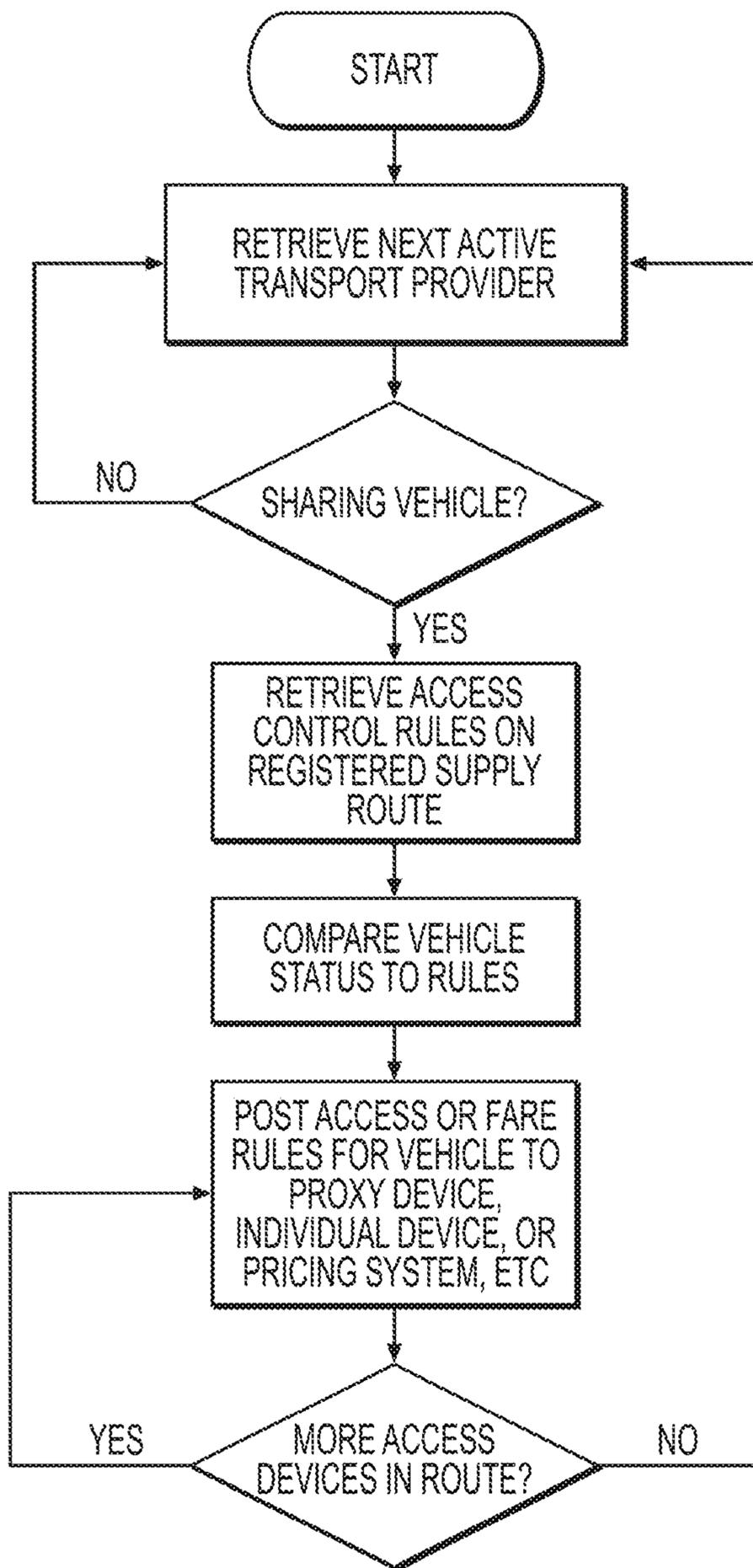
FIGURE 12c. ACCESS CONTROL SYSTEM, SERVER PUSH METHOD, CLIENT-SIDE LOGIC
