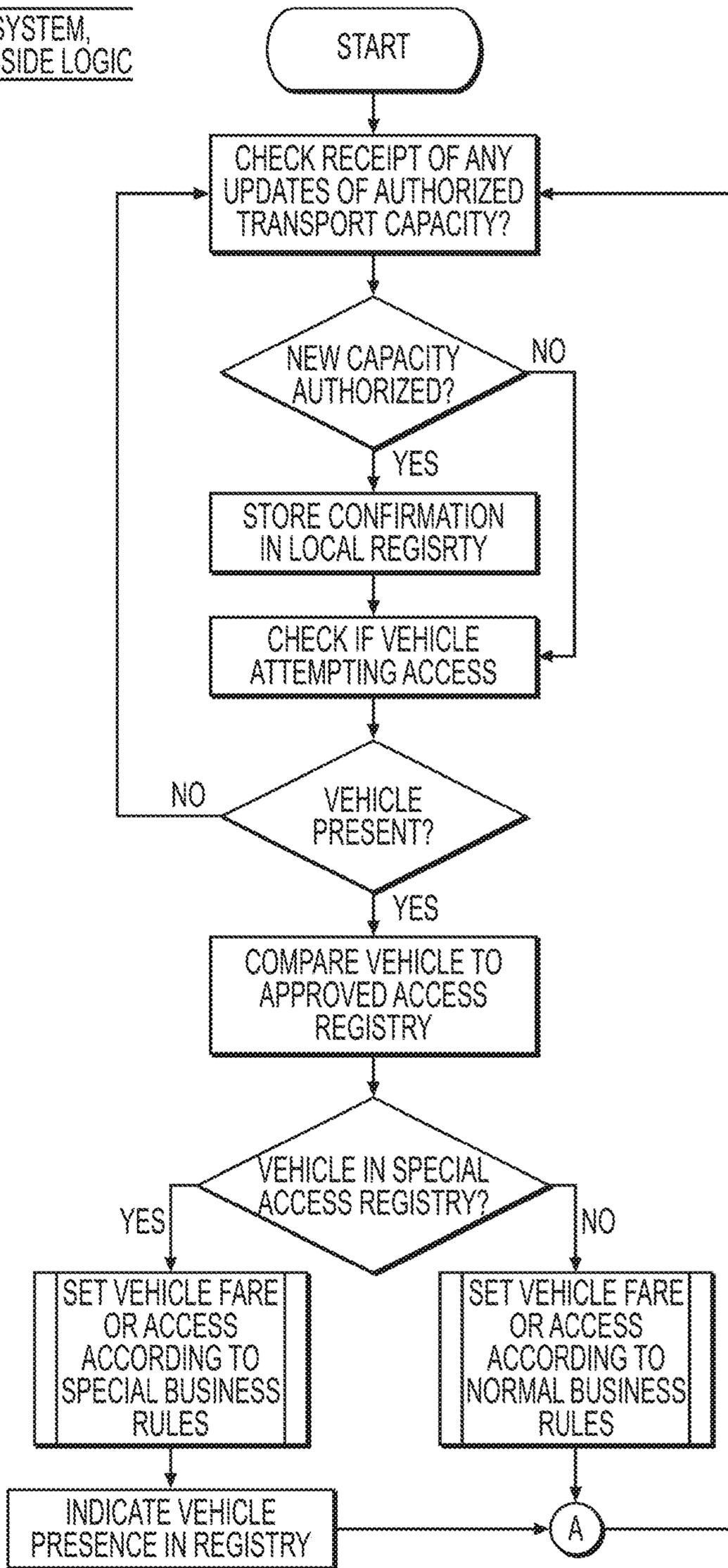
FIGURE 12d. ACCESS CONTROL SYSTEM, CLIENT PULL METHOD, CENTRAL SERVER-SIDE LOGIC
