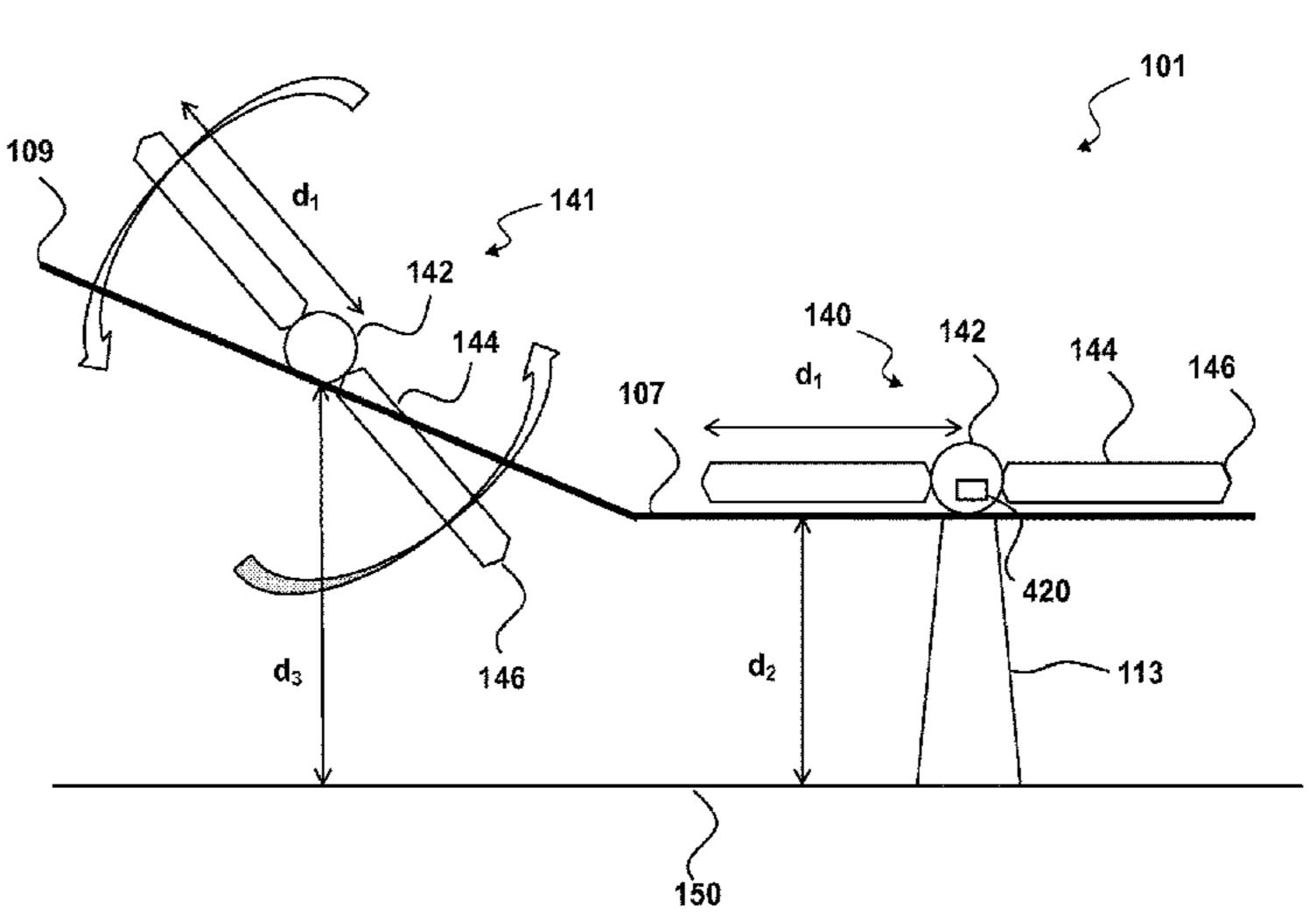
is held in an attitude that provides for clearance of the propeller blade to the ground upon landing.
