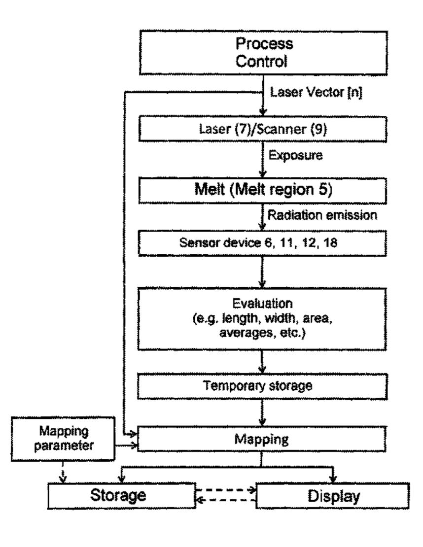
sensor values corresponding to the melt pool and/or the melt region. A visualization apparatus may display a representation of the three-dimensional component, with the display including the build coordinates and the sensor values in respect of a capture location thereof in the three-dimensional component. The displayed representation may be based on a display output that includes sensor values correlated with build coordinates.
