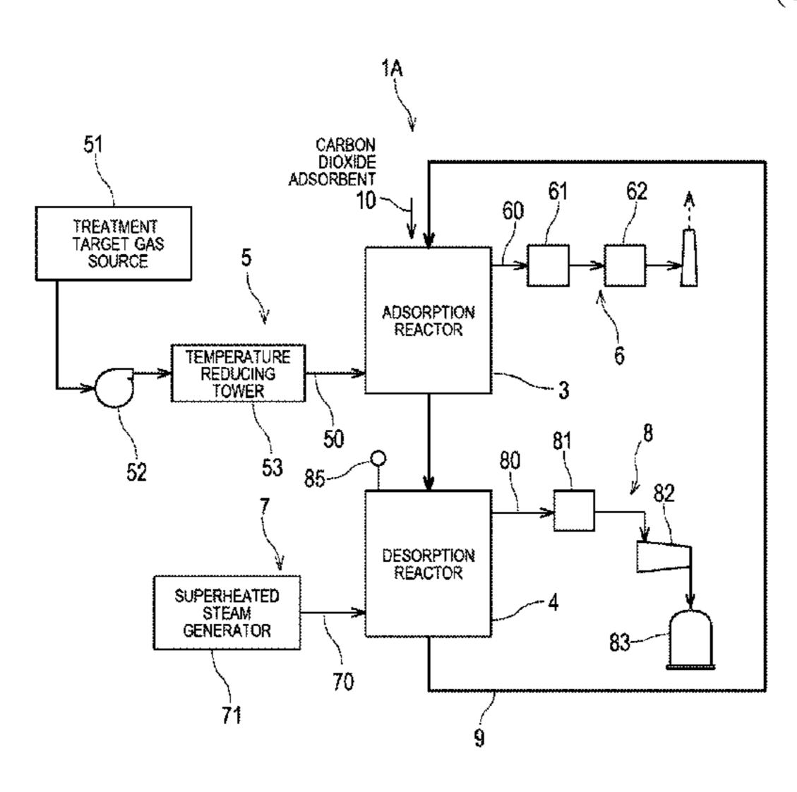
more than a temperature of the carbon dioxide adsorbent which contacts the superheated steam. The regenerated carbon dioxide adsorbent is utilized for adsorption of the carbon dioxide again without being subjected to a drying step.
