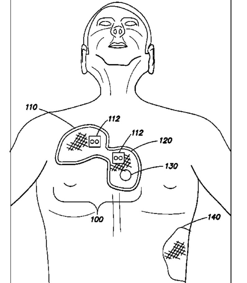
oriented in a first orientation and such that the CPR administration section is located above a sternum of a pediatric subject and the electrode section is located in a position appropriate for the administration of a defibrillation shock to the pediatric subject when the defibrillation electrode pad is oriented in a second orientation different from the first orientation.
