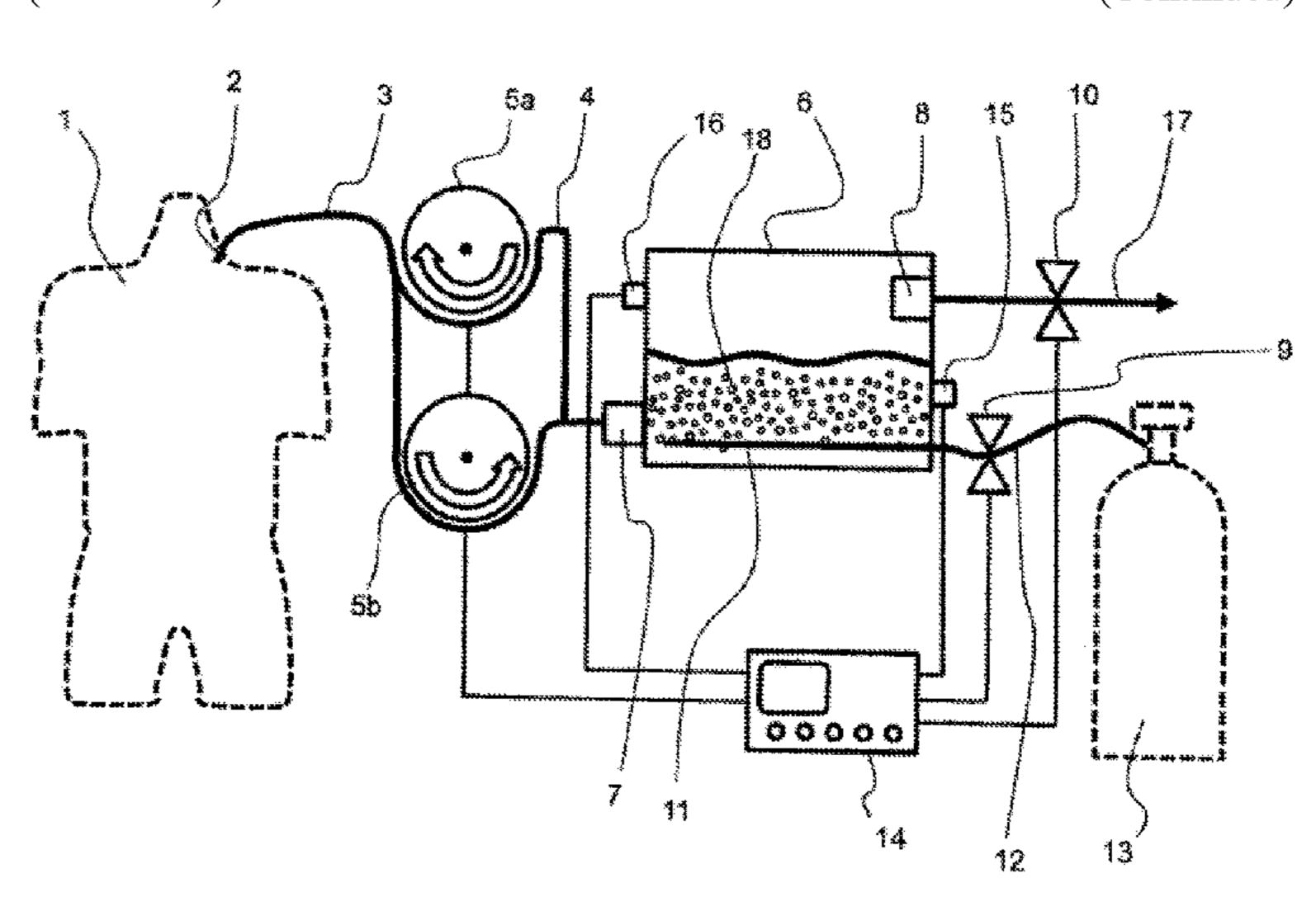
way of at least one pump into the gas exchange chamber, and to return the blood from the gas exchange chamber to the blood circulatory system of the person via the same first tube section.
