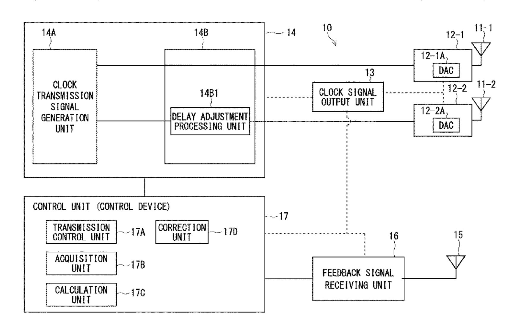
first correction value for correcting a first delay amount set value of a delay adjustment processing unit based on the first and second phase values.
