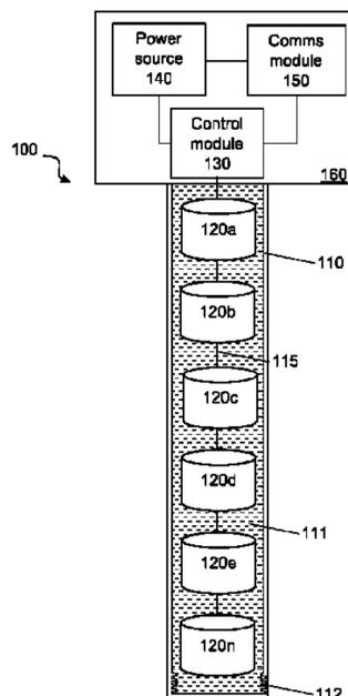
electrical signal associated with the temperature sensor modules to enable inference of the temperature of the resistive elements and the environment to which the tubing is exposed at the location of that resistive element.
