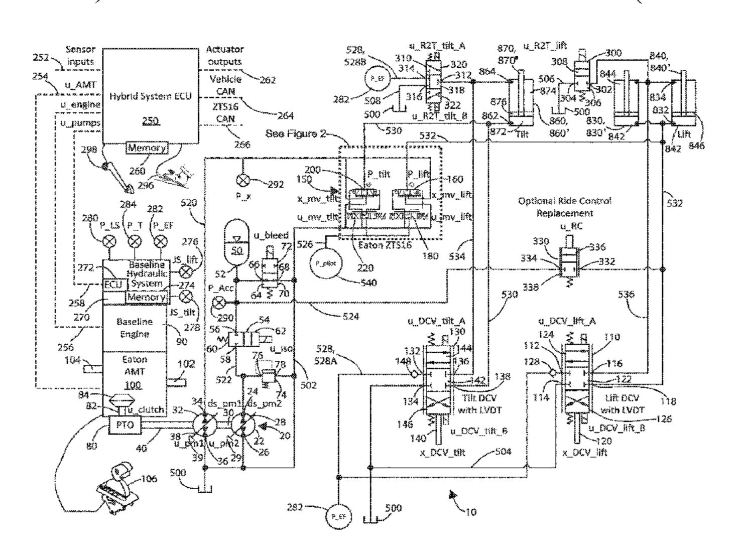
the power-take-off. The accumulator is hydraulically coupled to the second hydraulic circuit. The second hydraulic circuit is hydraulically coupled to a first rotating group of the hydraulic transformer, and a third hydraulic circuit is hydraulically coupled to a second rotating group of the hydraulic transformer.
