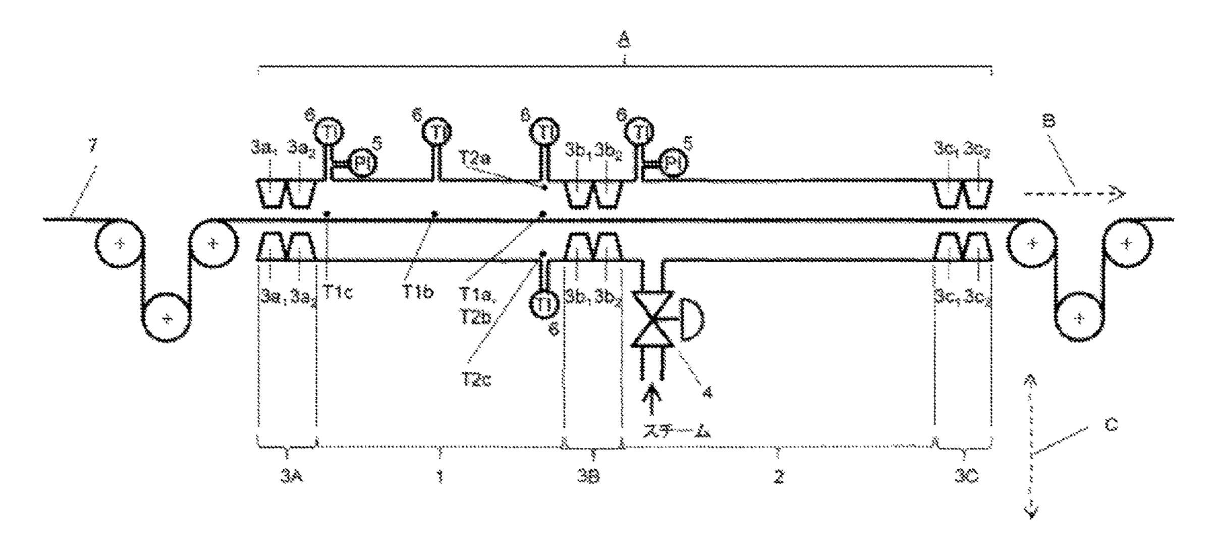
MPa, the heating zone is in a pressurized steam atmosphere at 0.45 to 0.70 MPa, temperature difference  $\Delta T1$  in the preheating zone of the steam drawing apparatus in the fiber bundle-moving direction defined in the specification is up to 5° C., and temperature difference  $\Delta T2$  in the preheating zone of the steam drawing apparatus in the cross-sectional direction of the steam drawing apparatus defined in the specification is up to 5° C.
