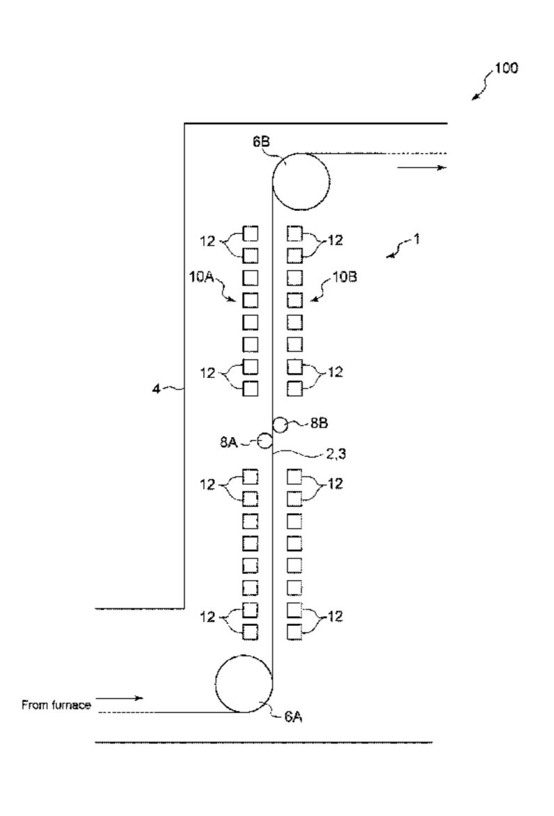
offset by a shift amount S from a center of the first nozzle in the width direction, and the center of the second nozzle is positioned in a region defined by an oval having a semi-axis of  $\Delta Xn/4$  in the width direction and a semi-axis of Yn/3 in the longitudinal direction. The shift amount S is expressed by  $S=m\times\Delta Xn/2$ , where m is an odd number such that S is closest to Xn/2.
