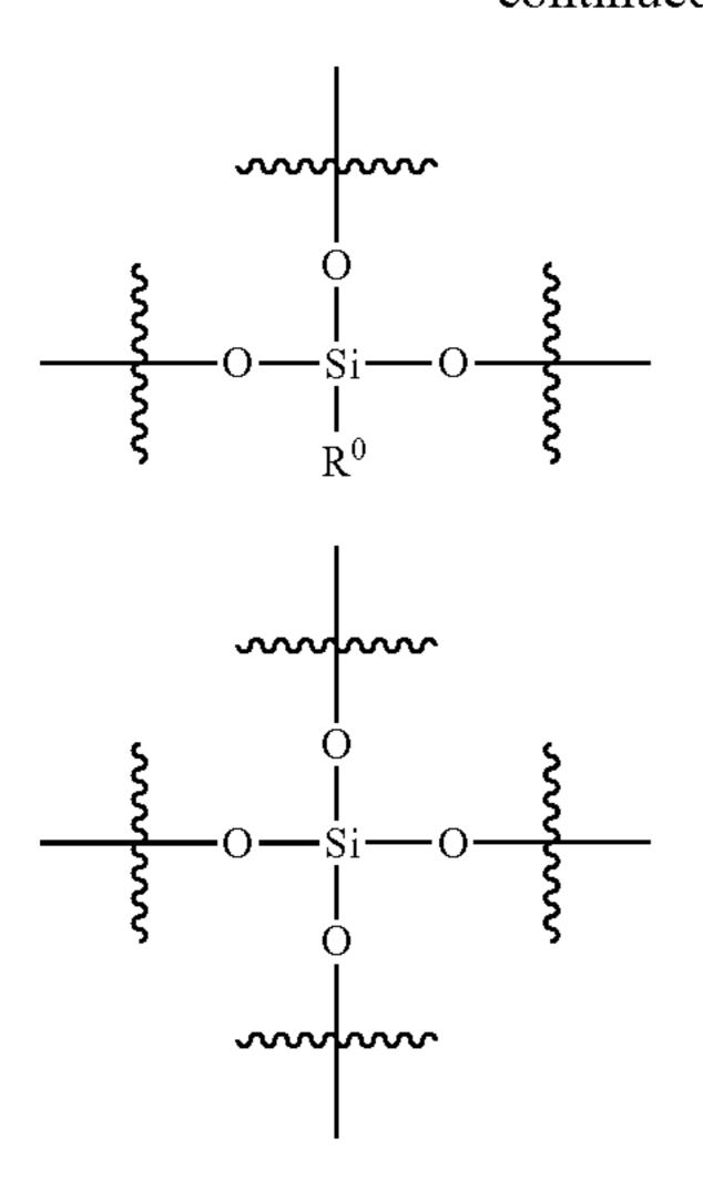
In these structures/formulae, each R<sup>o</sup> may be any hydrocarbon, aromatic, aliphatic, alkyl, alkenyl, or alkynl group.
