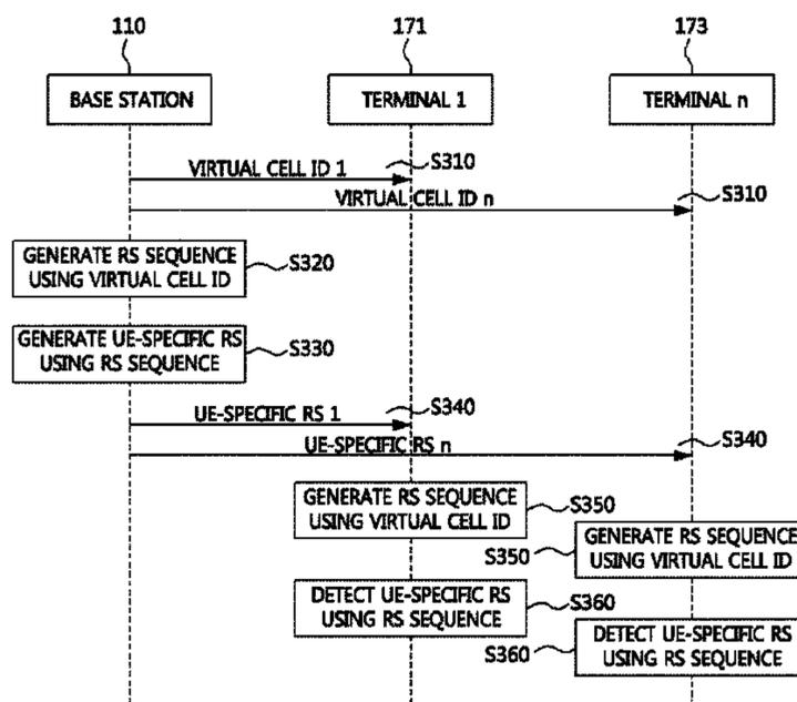
transmission signals by using the same physical layer cell ID or virtual cell IDs allocated to each terminal, and then the terminals generate uplink transmission signals by using the allocated virtual cell IDs.
