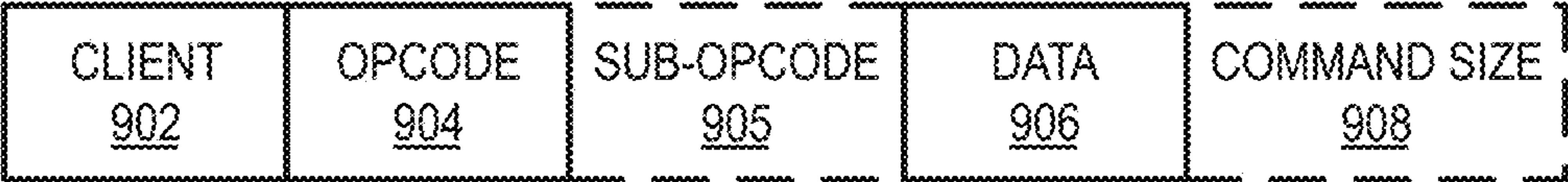
FIG. 9A GRAPHICS PROCESSOR COMMAND FORMAT 900
