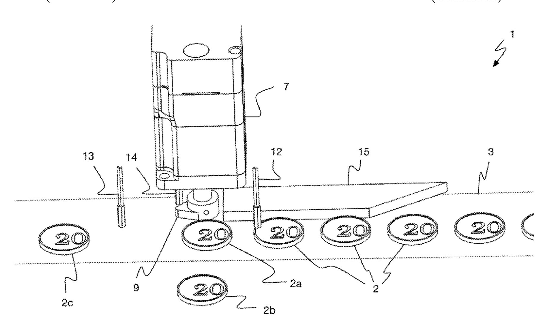
object to be discharged from the conveyor path. During the sorting of good parts and defective parts, only the conveyed objects which have been classified as good parts in accordance with the classification system are discharged by means of the diversion element.
