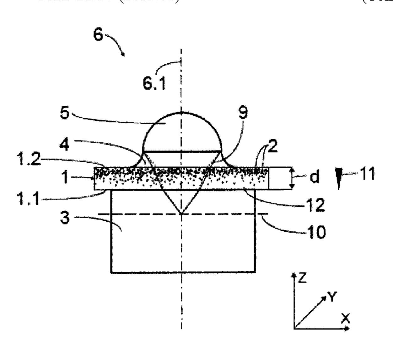
specimen delimiting element, and has at least one gradient portion in which no porosity is present, such that a separation of a specimen medium on one side surface of the specimen delimiting element and an immersion medium on an opposite side surface of the specimen delimiting element is effected by means of the specimen delimiting element. The invention furthermore relates to a microscopy method and to a microscope using the specimen delimiting element.
