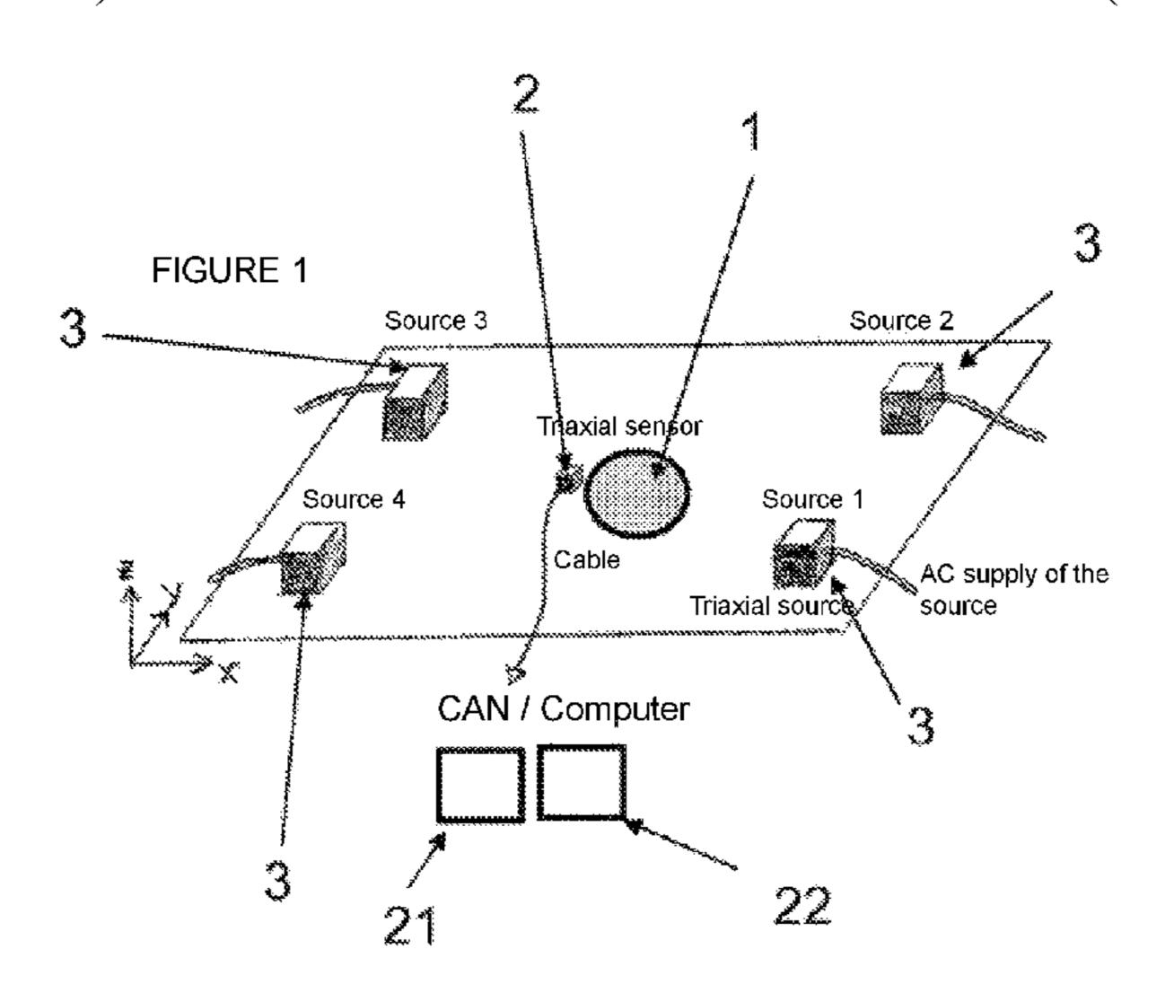
generators (3) said selected sub-set of the set of generators (3) including each generator (3) for which said estimated parameter is less than at least one reference threshold;
