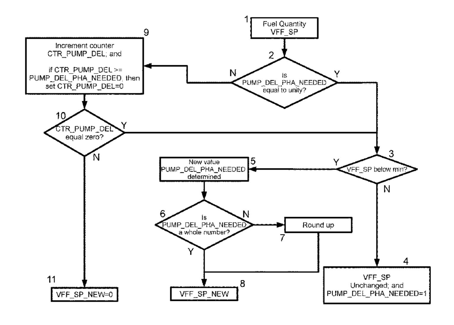
subsequently disabling the fuel pump for a number of occurrences of the set amount of fuel equal to the number of compressions of a volume equal to the set amount of fuel to be compressed.
