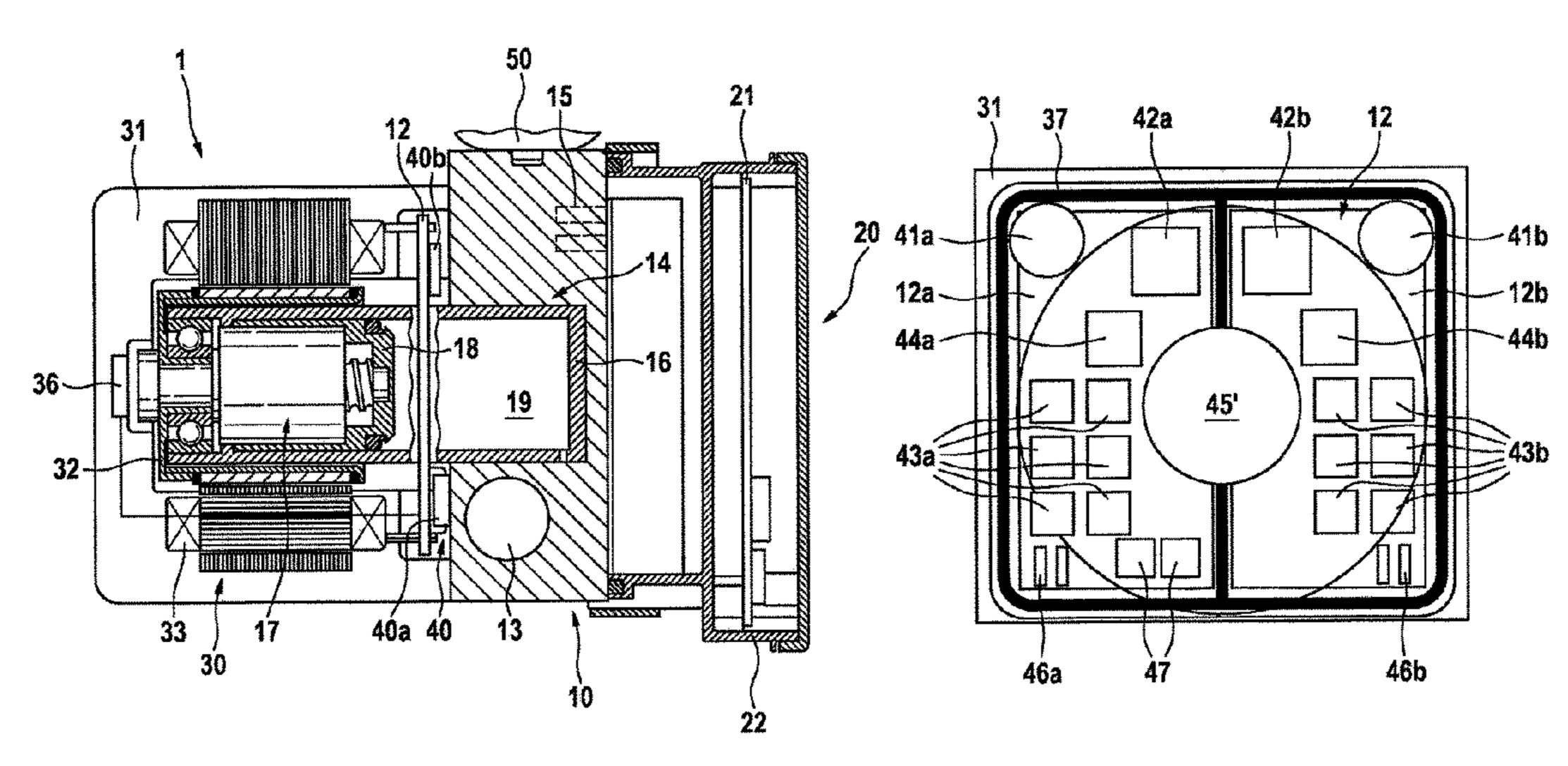
control unit which includes a first printed circuit board with electric and/or electronic components for actuating the valves, and an electric motor for driving an electrically controllable, hydraulic pressure source, wherein electric and/or electronic components, in particular power electronics components for actuating the electric motor are arranged on a second printed circuit board which is arranged separately from the electronic control unit.
