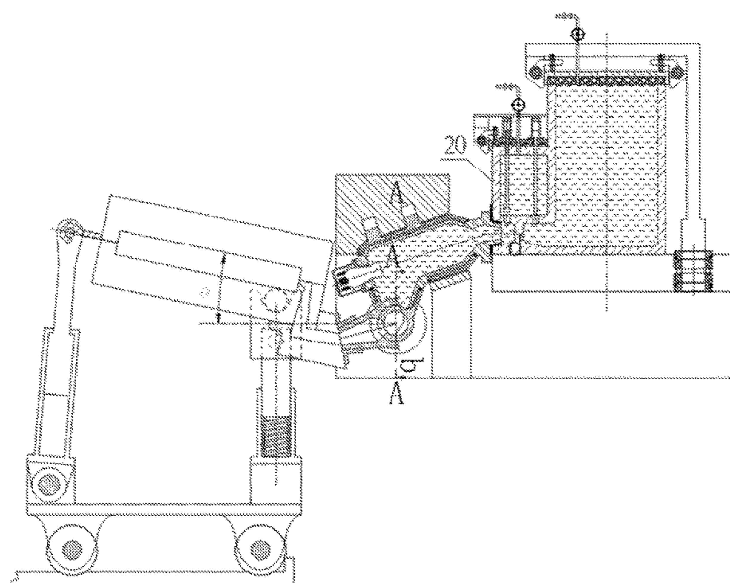
the top of the pressure supplying cylinder. A liquid inlet of the crystallization treater is communicated with the pressure supplying cylinder while a liquid outlet is communicated with the pouring system and the mold cavity. The crystallization treater is provided with a grain refining mechanism.
