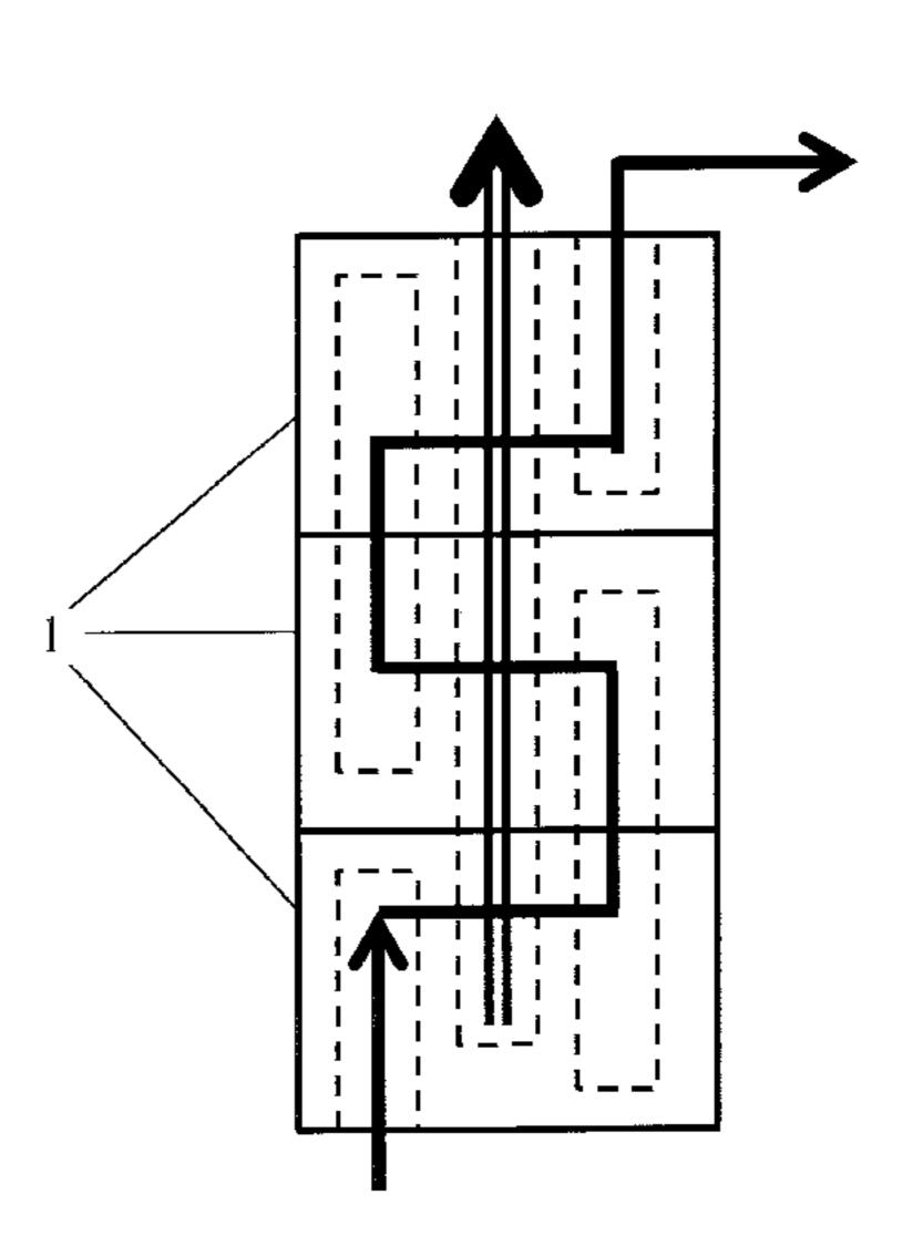
flow filtration (TFF) system, recovering permeate and a portion of the retentate from the system in separate containers without recirculation through the TFF system, and recirculating the remainder of the retentate through the TFF system at least once. The methods can be performed using an SPTFF or a TFF system that comprises manifold segments to serialize the flow path of the feed and retentate without requiring diverter plates.
