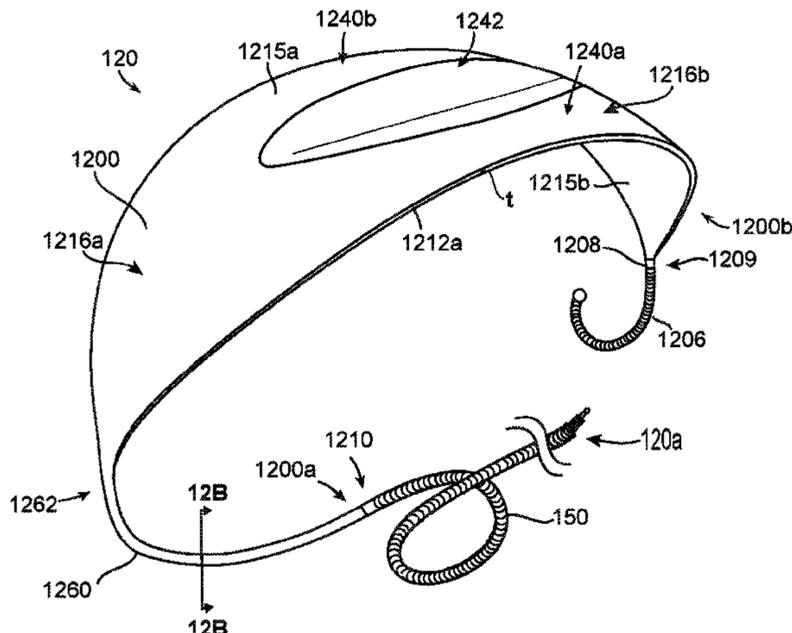
across at least a portion of one or both of its length or its width. The mesh is configured to be positioned within the aneurysm in the deployed state such that the mesh extends over the neck of the aneurysm.
