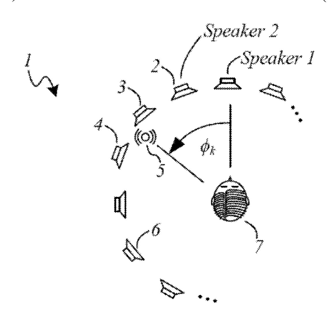
function involves smoothing the discrete panning function, and determining a rendering operation for converting the audio signal in the intermediate signal format to the set of speaker feeds, based on the target panning function and the spatial panning function. The present disclosure further relates to a corresponding apparatus and a corresponding computer-readable storage medium.
