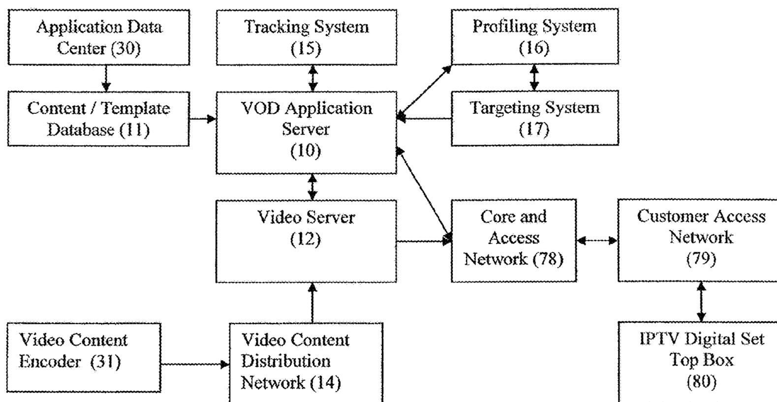
Figure 3: VOD Content Delivery System, Overall Architecture for IPTV System
