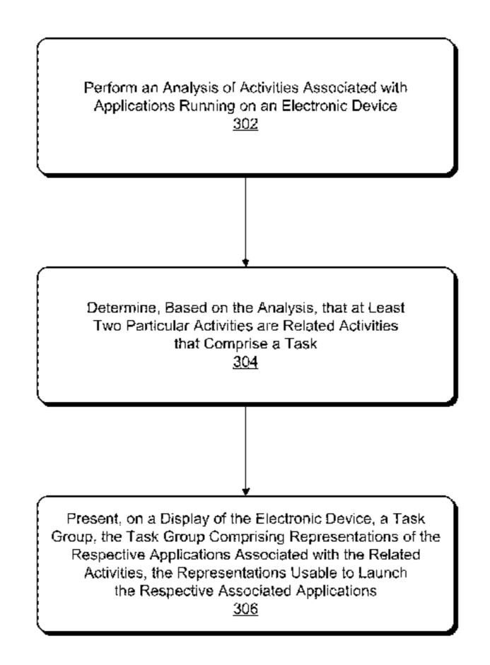
ager can automatically determine that the activities and actions represent a task and display a task group that includes the applications that represent the task. The task groups may be visually displayed as a stack, strip, or pile of windows or thumbnails representing each application or other content the person could use for the task.
