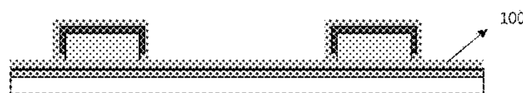
3) INJECT CHARGED INK AND LAMINATE FILM
