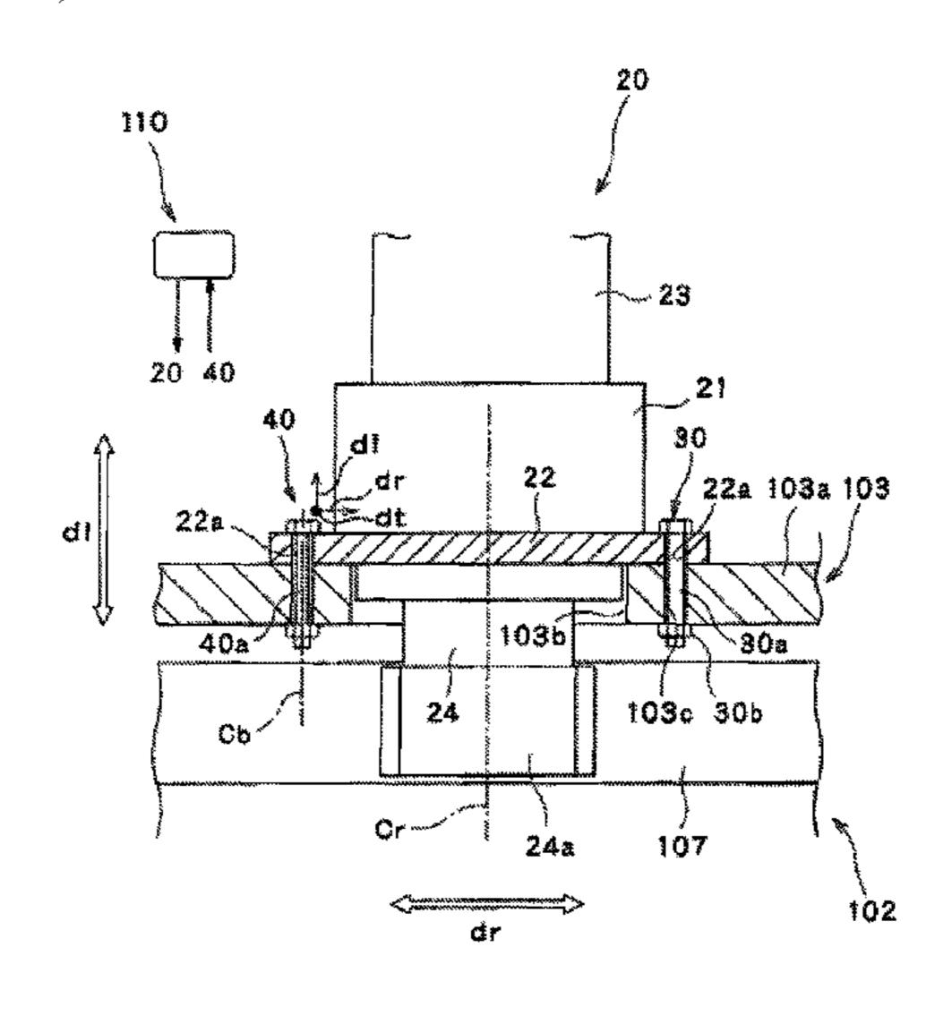
wind turbine. The sensor measures a change in installation state of the driving device body with respect to the one structure.
