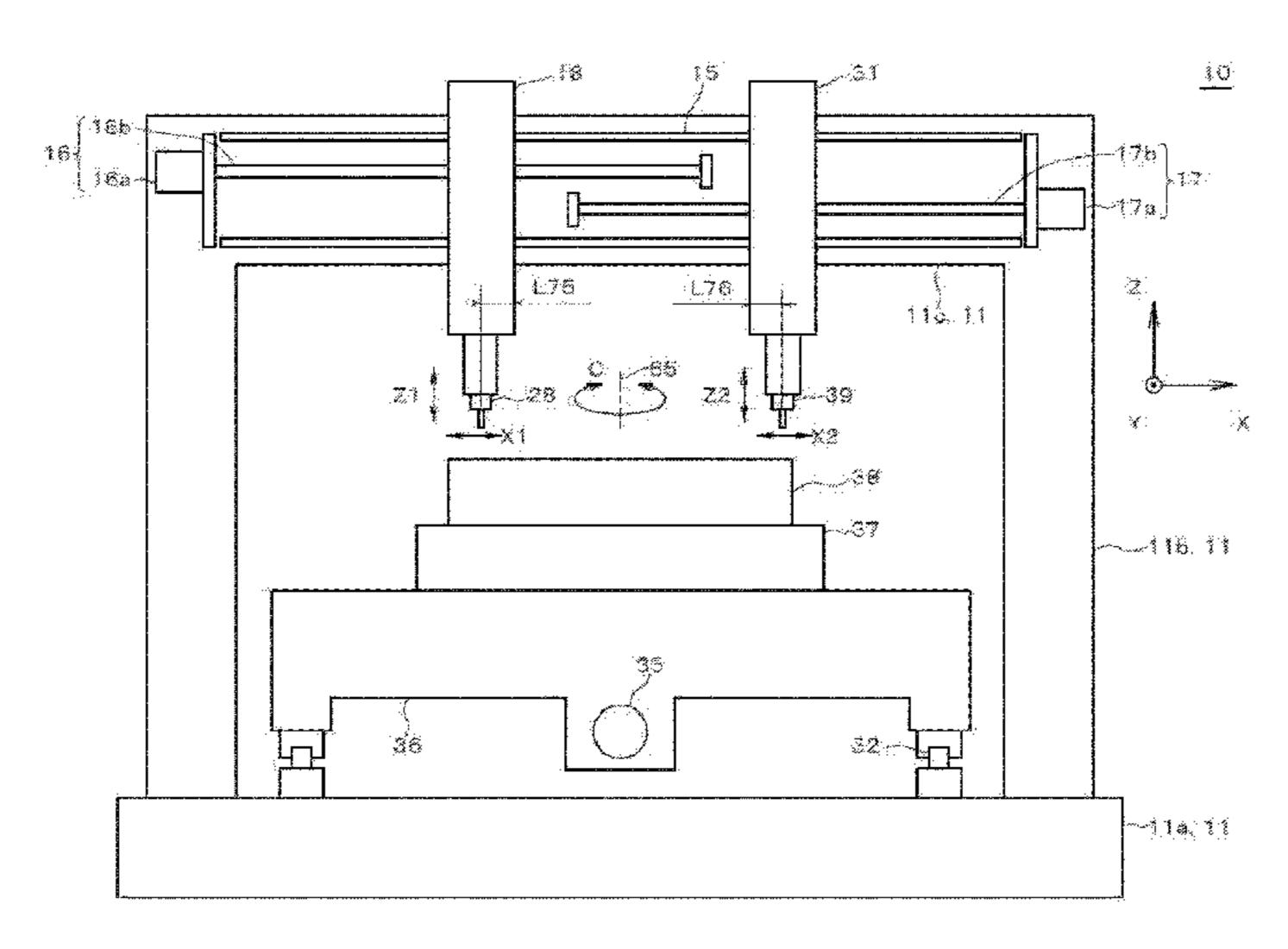
aligned; and machining the first hole with the first spindle and the second hole with the second spindle.
