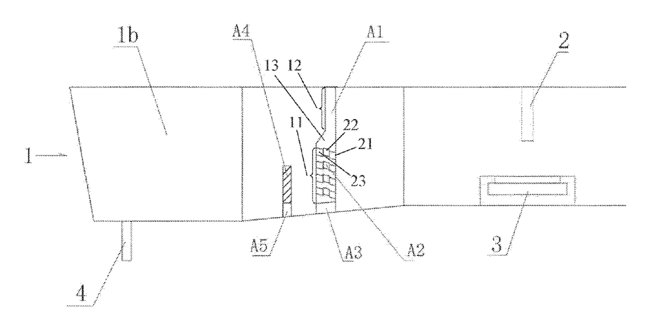
flows into the pouring zone cavities and then flows out from the discharge ports. The flow-controllable tundish structure has the advantages of a simple structure, easy building and lower cost, and has a good liquid steel purification effect.
