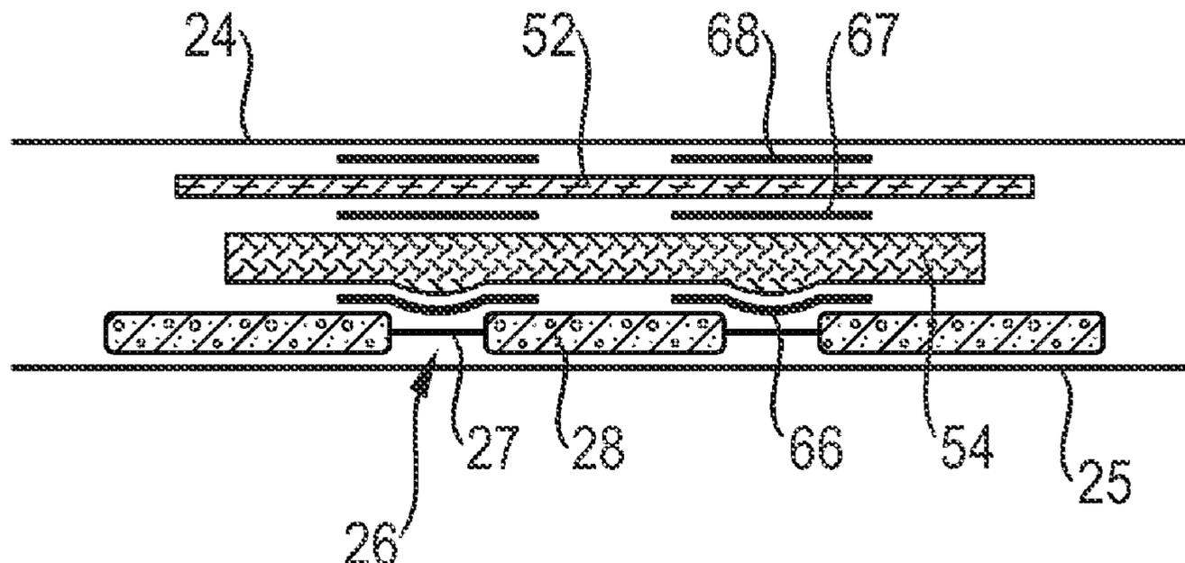
of the core wrap in the area substantially free of absorbent material. When the absorbent material swells, the core wrap forms one or more channels along the area substantially free of absorbent material. The formation of the channel in the absorbent core causes the formation of one or more corresponding ditches in the fibrous layer.
