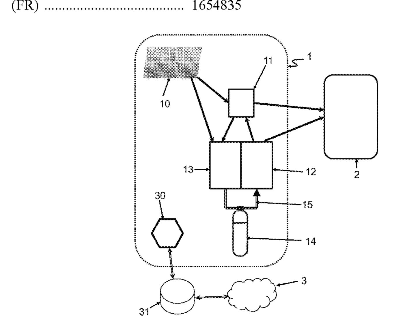
of the stability of the power balance during a safety period; controlling the fuel cell and the electrochemical unit: to activate the electrochemical unit if the power balance is greater than a first threshold and the data are not characteristic of a subsequent decrease in the power balance; activating the fuel cell if the power balance is less than a second threshold, which is less than the first threshold, and the data are not characteristic of a subsequent increase in the power balance.
