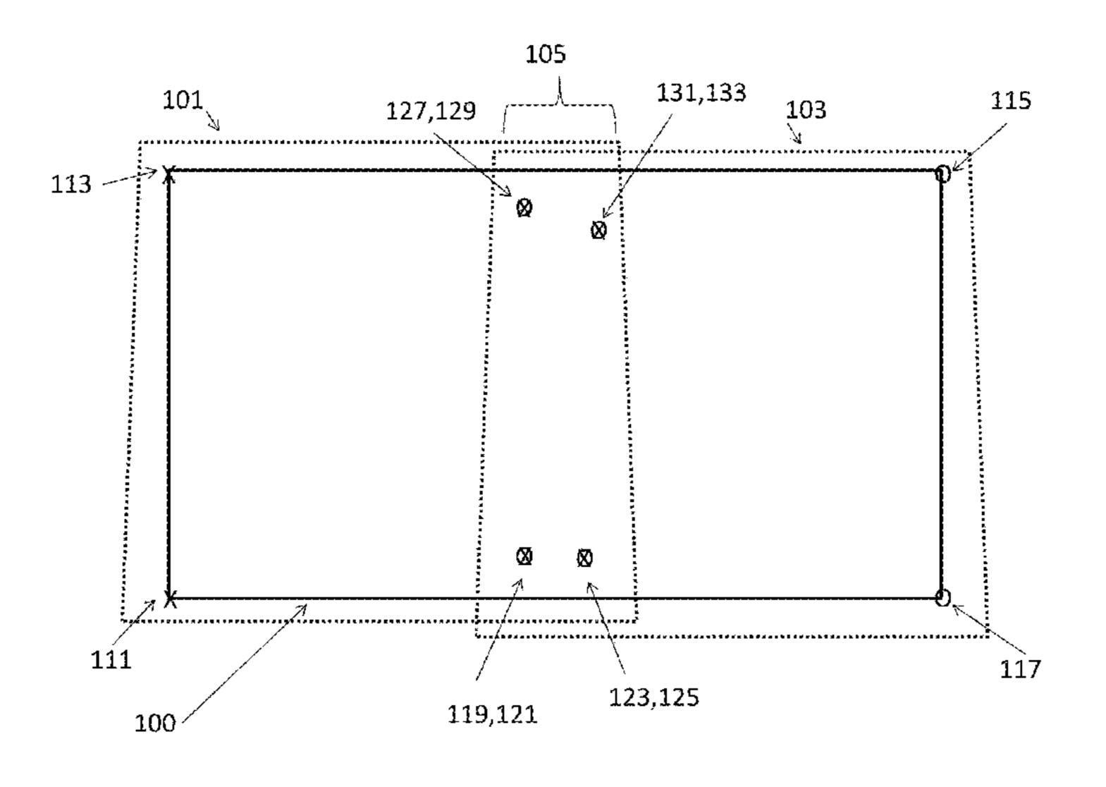
points on each projector, and avoiding selection of precisely measured screen points. The system conversely finds correspondences between projectors, allowing mapping of the projectors into a common coordinate system, and quick warping of the coordinate system to the screen.
