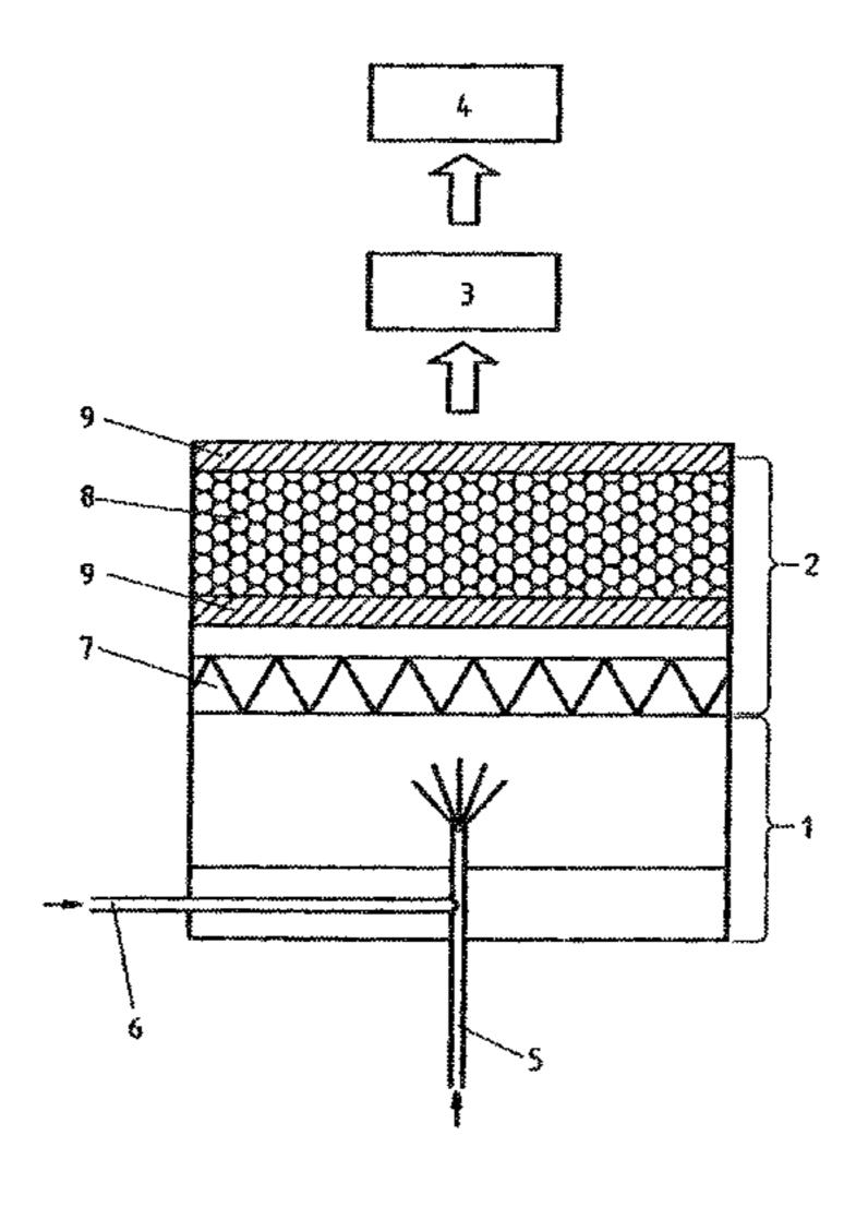
from step (d) to form synthetic quartz glass. The cleaning device includes a bulk of porous silica particles which have a BET specific surface area of at least 2 m<sup>2</sup>/g. A device for carrying out the method is also provided.
