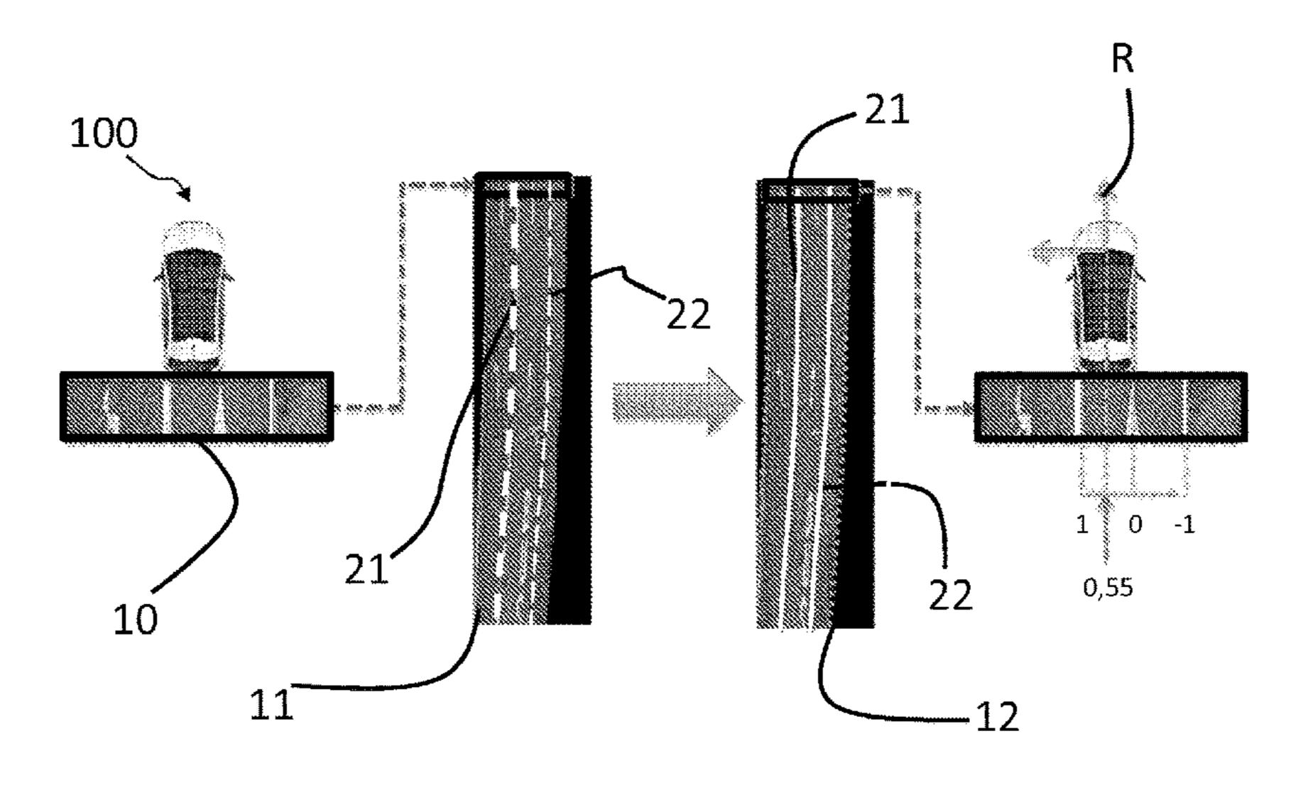
positions of the vehicle, —the determination of an estimated attention level of the driver at a past instant t3, as a function: o of the evolution of the lateral position of the vehicle, o of the analysis of the profile of a road portion at least partially situated upstream of the vehicle at the instant t3.
