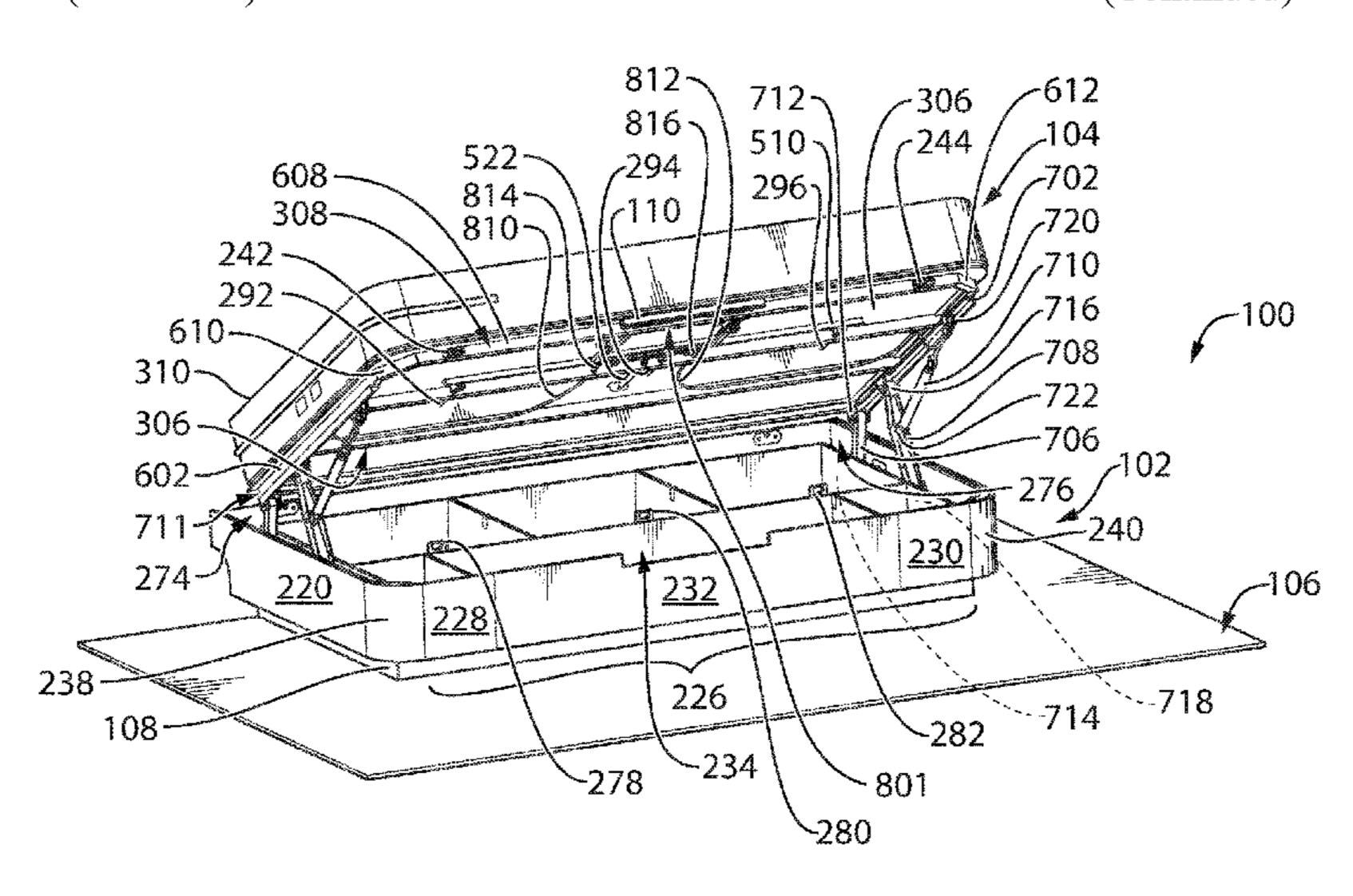
lock actuator (801) is in the actuated position. The locking assembly locking the top (104) in the open, closed, or an intermediate position when the lock actuator (801) is in the released position. The latching actuator (110) and the lock actuator (801) are operatively connected to the top (104) and move with the top (104) between the closed and the opened position.
