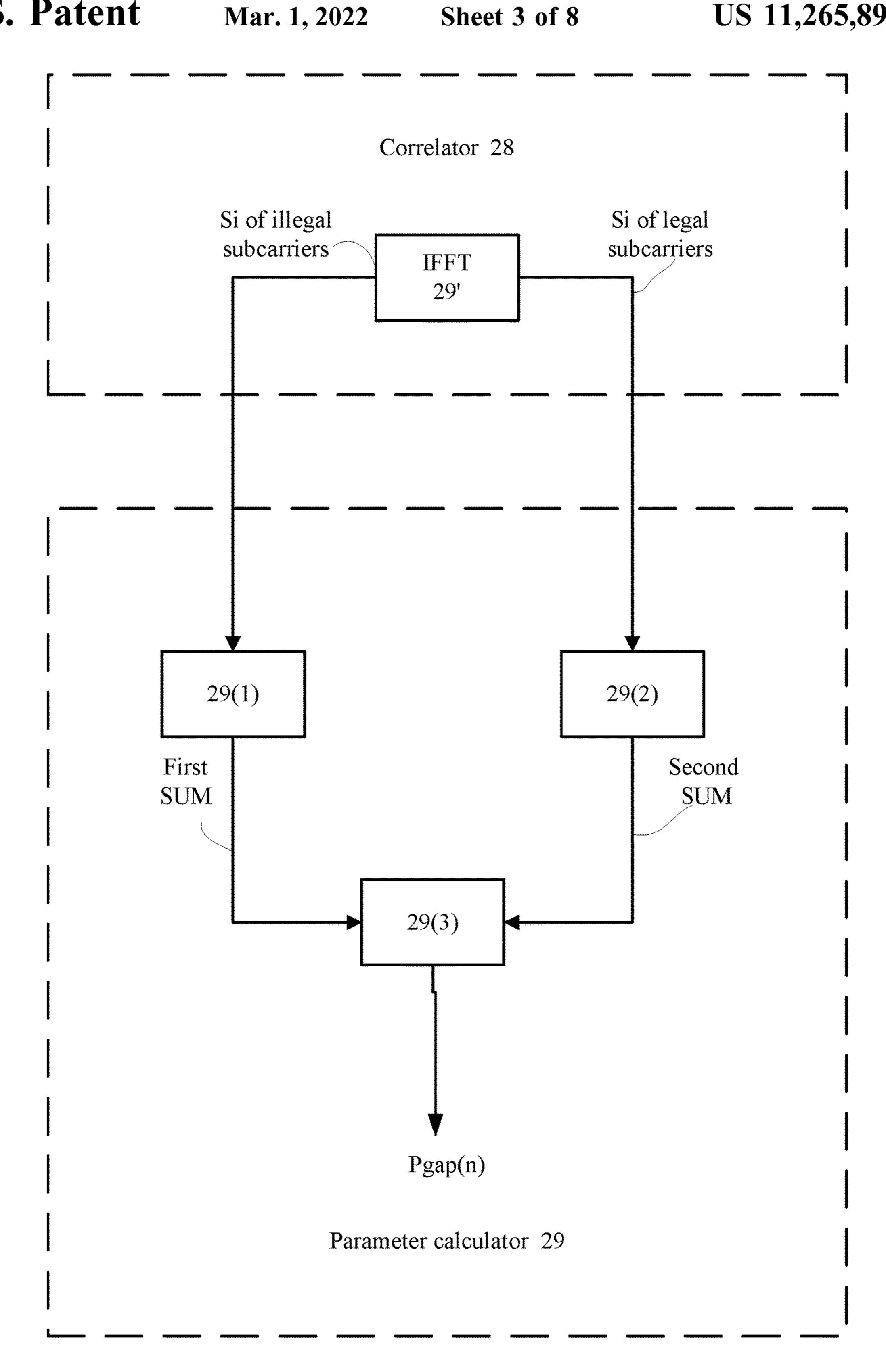
Receiving, by a skywave propagation receiver, received signals that are within a skywave frequency range that comprises legal subcarriers and illegal subcarriers. 110
