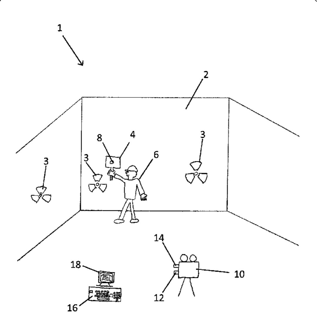
of the handheld probe, when the handheld probe (4) is determined to be less than a threshold distance from the surface (2) being surveyed.
