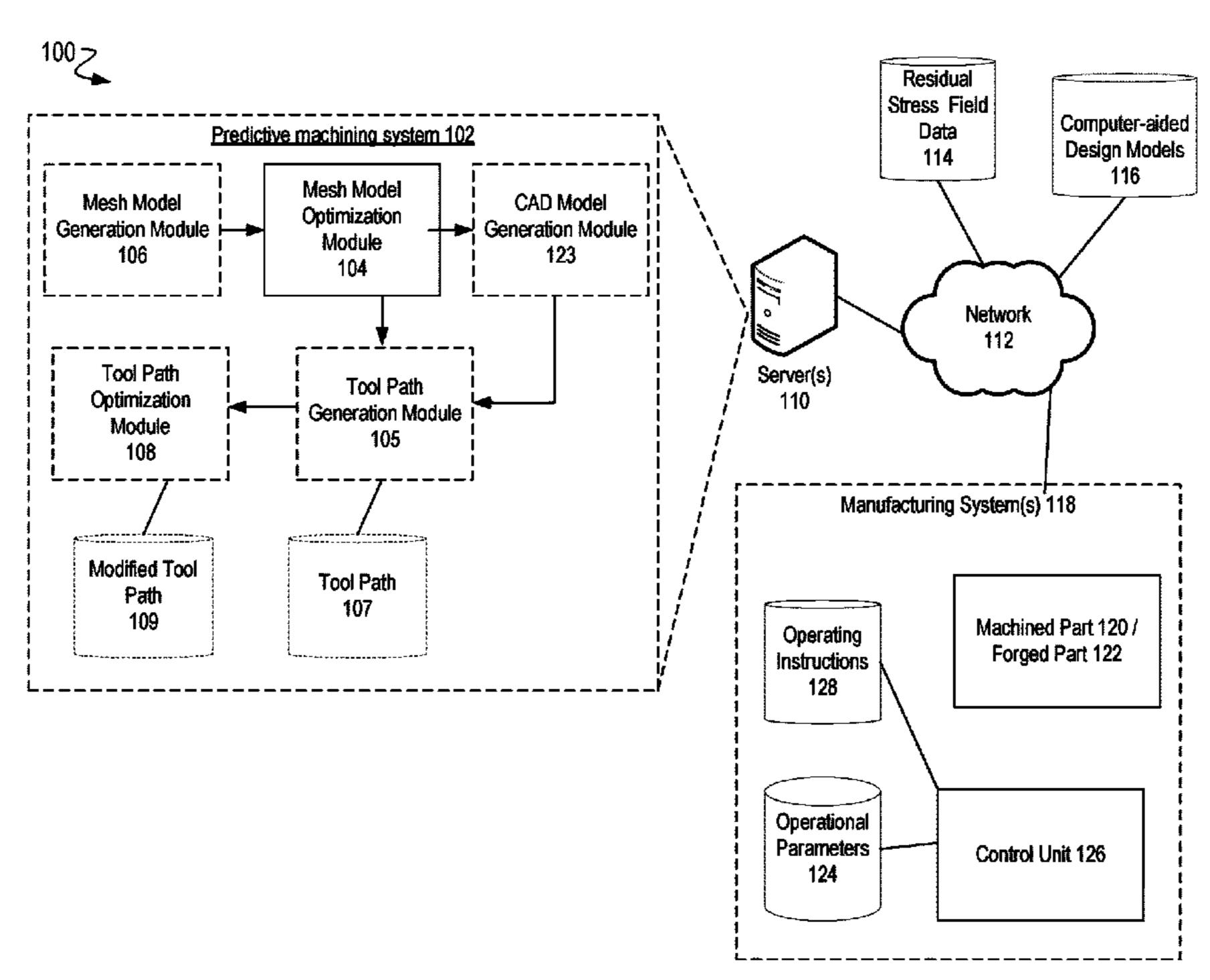
machined part, updating the mesh model by applying the residual stress field data to the multiple nodes corresponding to the at least one boundary to change positions of the multiple nodes in the mesh model, repeating the updating until an amount of change to each of the positions of the multiple nodes in the mesh model satisfies a correction criteria, and providing the compensated mesh model for use in machining the machined part from the forged part.
