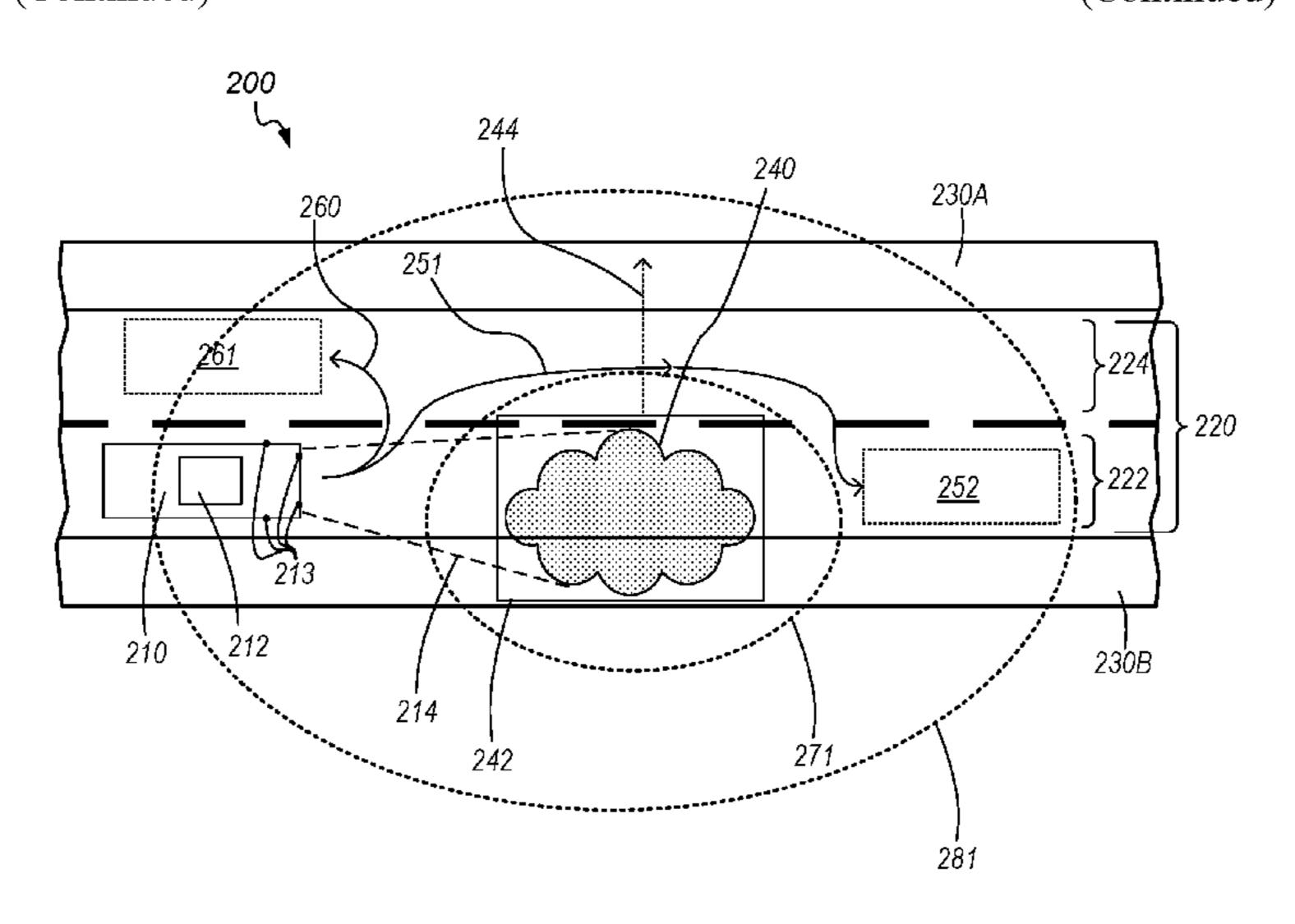
according to avoidance driving parameters to avoid non-solid objects, and a navigation system may characterize a non-solid object as a solid object having dimensions and position which encompasses the non-solid object, so that the vehicle is navigated in avoidance of non-solid objects as if the non-solid objects were solid.
