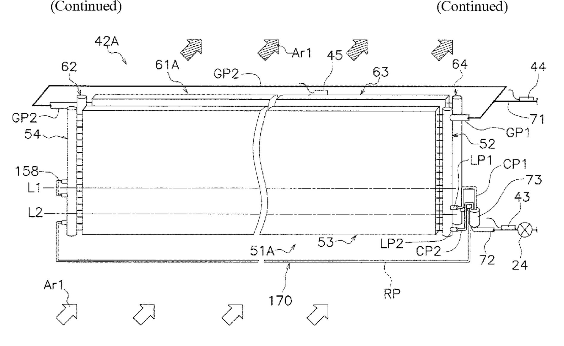
second resistance to refrigerant flow in the downstream heat exchange unit are adjusted in order that the degree of superheating of refrigerant at the downstream refrigerant outlet is smaller than the degree of superheating of refrigerant at the upstream refrigerant outlet.
