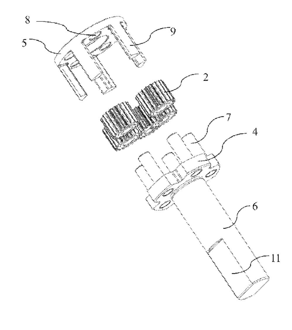
rotating circumferentially relative to the disc portion. The planet carrier assembly according to the present application has the advantages such as low cost, high strength, and simple assembly.
