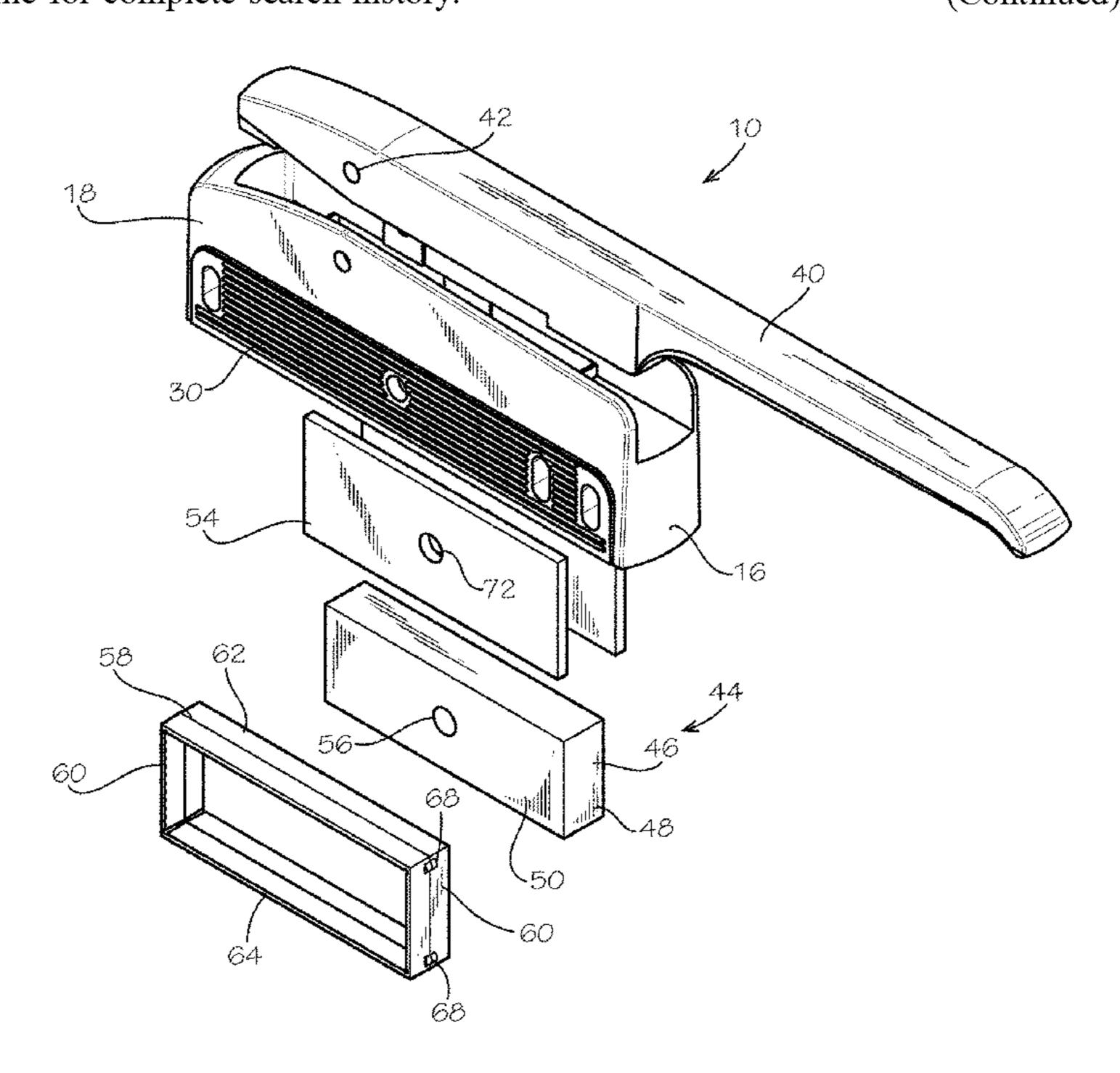
peripheral edges of the magnet. The peripheral sleeve is generally rectangular in shape having two oppositely disposed end walls (60) which include a cushioning projection (68). A pivot pin (74) extends through the magnet assembly to allow rocking motion.
