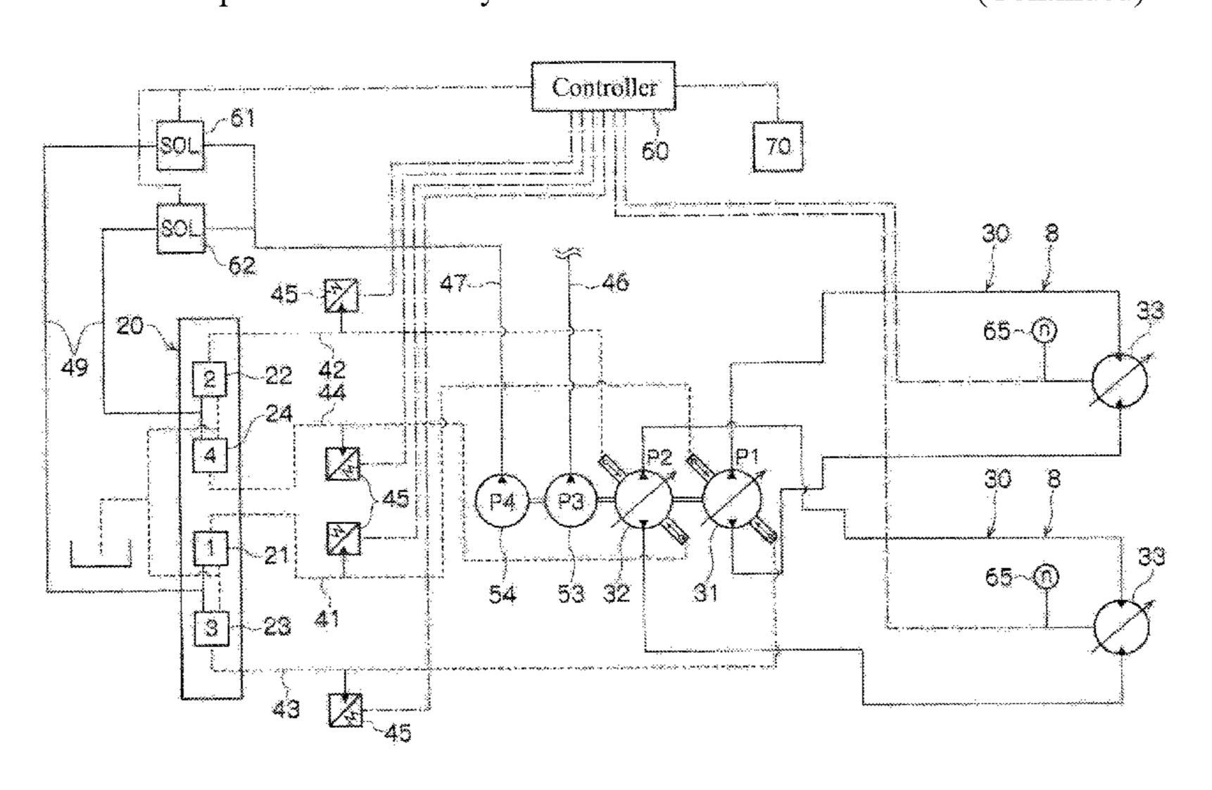
operation of the remote control valve (21, 22, 23, 24), on the basis of a setting signal, a pressure signal, and a rotation speed signal. The remote control valve (21, 22, 23, 24) controls a flow rate of the hydraulic oil discharged from the pump (31, 32) by changing or keeping constant the pressure inside the pilot line (41, 42, 43, 44).
