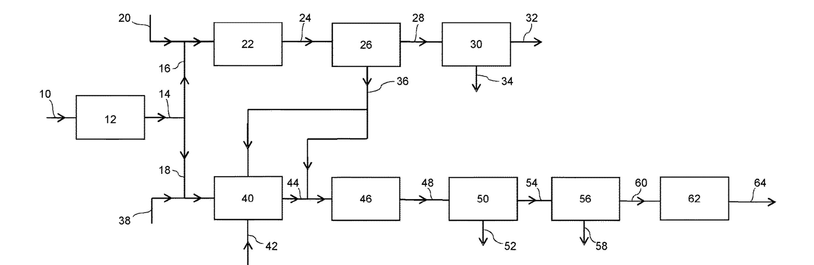
process gas comprising the first synthesis gas stream, and (d) synthesising ammonia from a second process gas prepared from the second synthesis gas stream, wherein a purge stream containing hydrogen is recovered from the methanol synthesis step (c) and a portion of the purge gas stream is fed to the autothermal reformer and/or the second synthesis gas in step (b).
