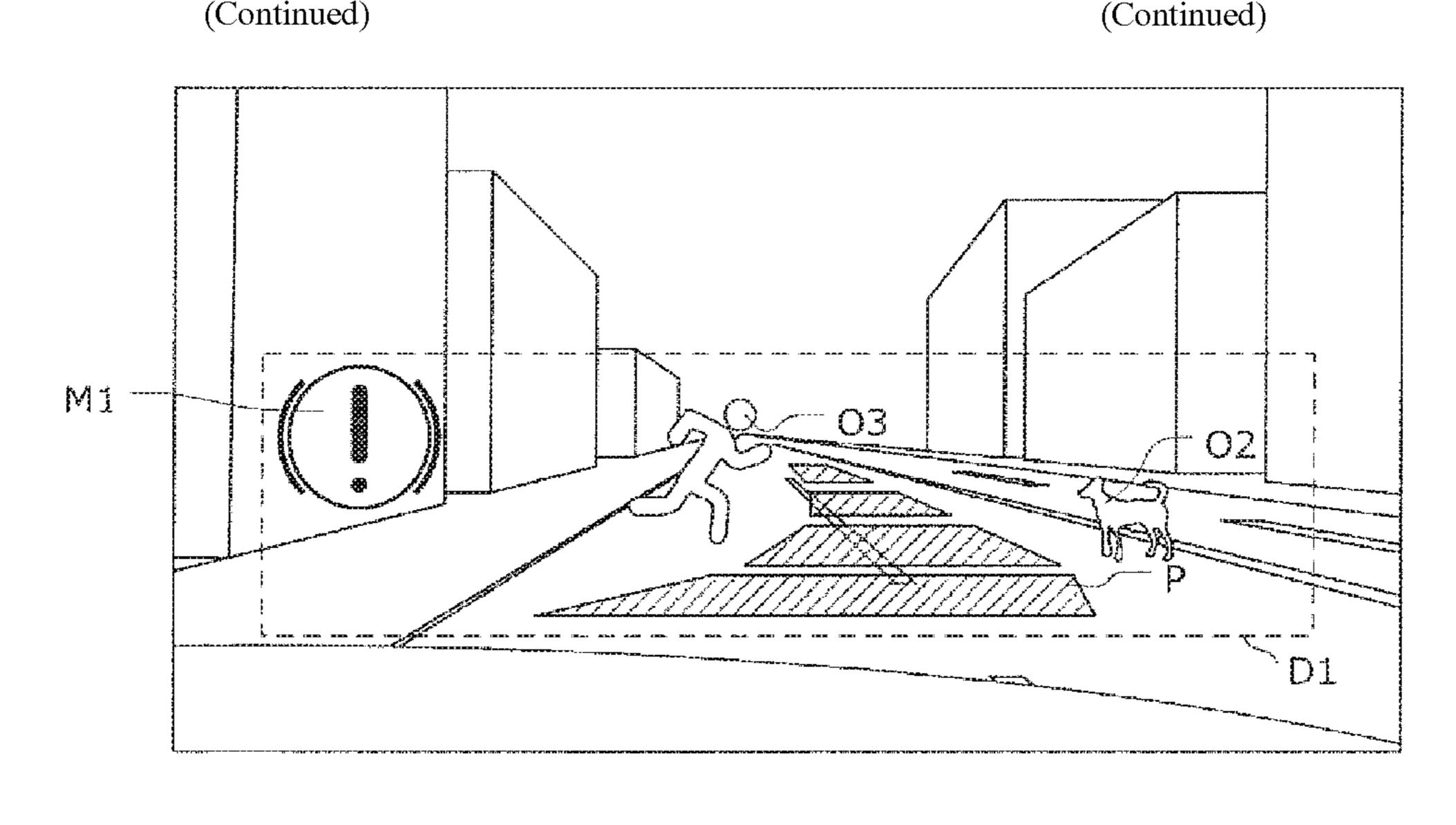
an avoidance path for avoiding the contact, based on the position relevant information and the vehicle information. The information display displays the avoidance path.
